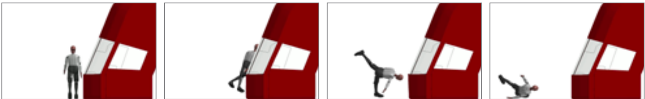
Future buses will have a more sloped windscreen and more rounded corners to help deflect pedestrians more upwards and laterally to reduce run-over risk.
