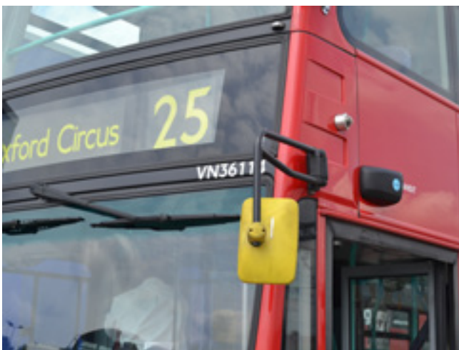
Additional sensors on buses can help to detect cyclists in blind spots.
