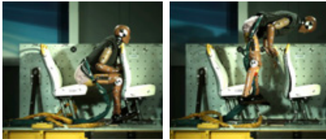
Passenger is poorly restrained.
