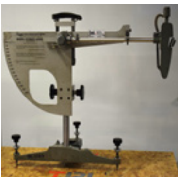
The Portable Skid Resistance Tester (PSRT).
