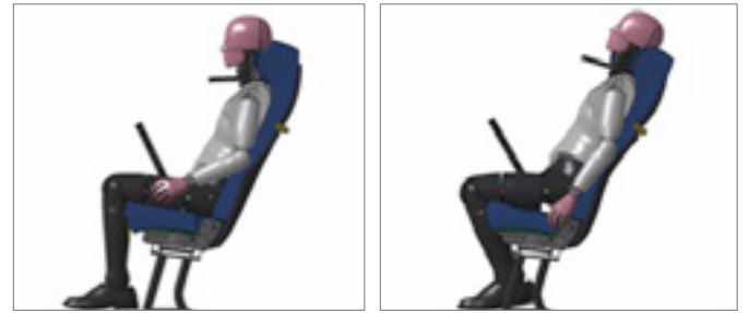
High back reduces neck extension when rear facing.
