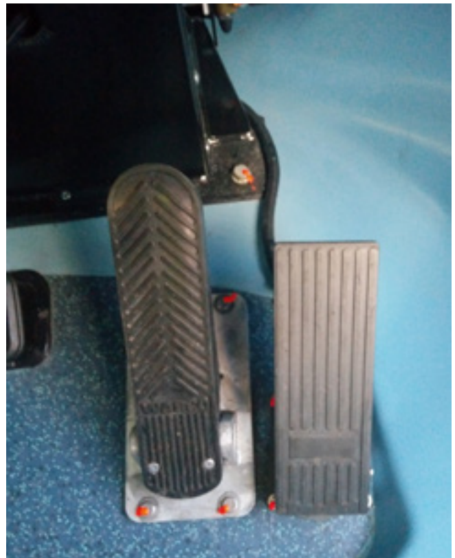
Pedal application error is a rare but high risk event when the accelerator is pressed instead of the brake pedal.
