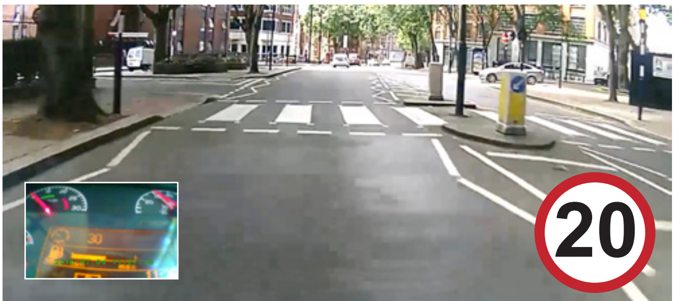
Intelligent Speed Assistance (ISA) supports the driver with keeping to the speed limit.
