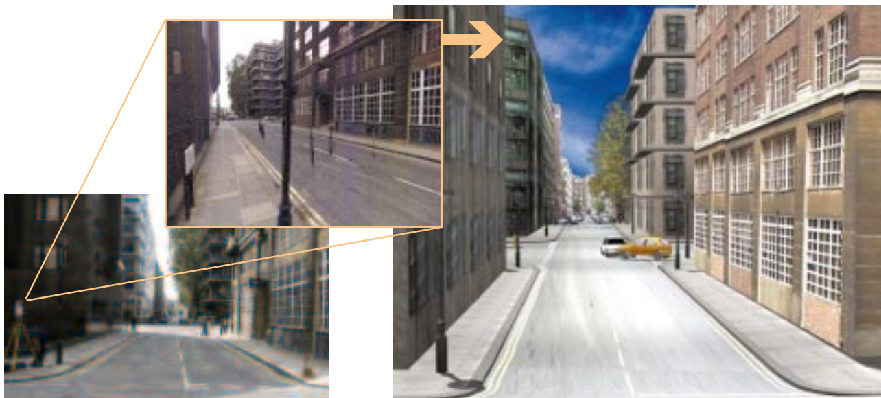
What the technology can do—scanner collects survey data to produce 3D scan. Scan is used to build 3D environment for visualisation of accident reconstruction
