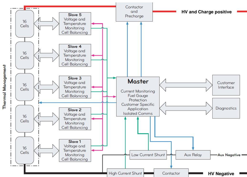
Figure 30. Schematics of a typical BMS. The figure originally provided by and reproduced with the permission of Johnson Matthey / Axion, it is the copyright of Johnson Matthey Battery Systems [2]<sup>44</sup>
