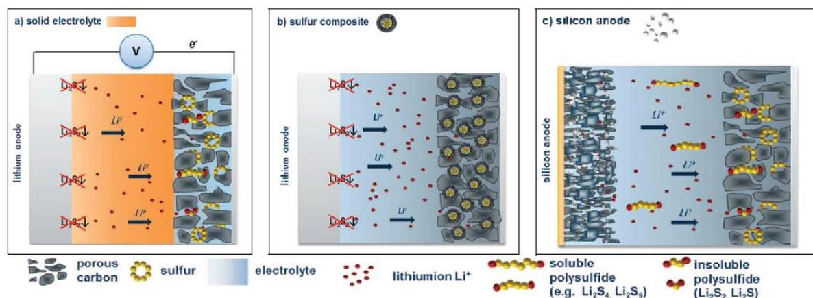
**Figure 8. Different Li-S battery configurations to overcome limited cycle life: a) use of solid electrolyte, b) encapsulated sulphur particles, c) silicon anode (shown under discharge) [43]<sup>22</sup>**
