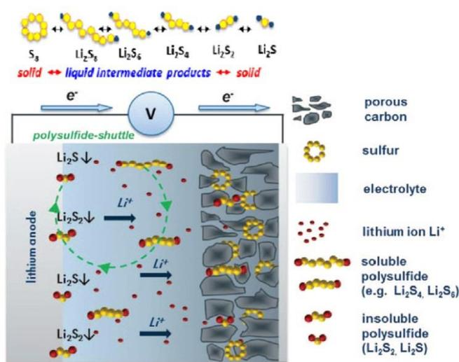
Figure 7. Li-S cell scheme and reactions taking place within it, under discharge [43]<sup>18</sup>
