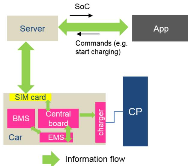
Figure 36. Typical communication flows between the car and the EV owner
