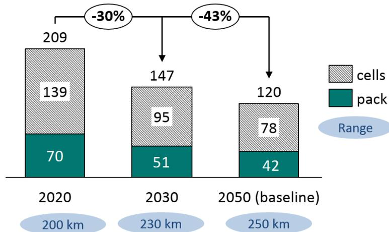
Figure 24. Total future pack mass split (kg) between cell and pack components (30kWh pack, NMC cathode, baseline scenario)<sup>37</sup>
