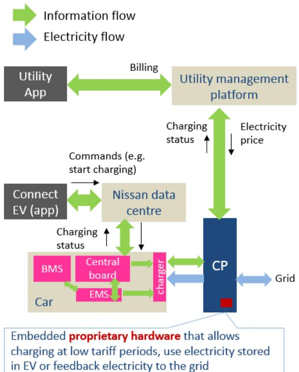
**Figure 39. Vehicle to Grid service schematics developed by Nissan and Enel**
