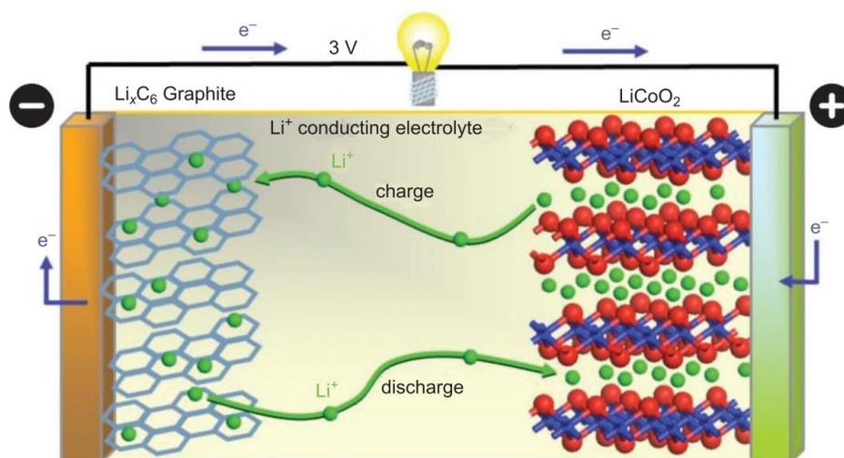
**Figure 2. Working mechanism of a typical lithium cell (intercalation: reversible insertion of the lithium ion into the electrodes), showing the electron flow under discharge and lithium ion flow under both charge and discharge. The figure originally provided by and reproduced with the permission from Johnson Matthey / Axion and is the copyright of Johnson Matthey Battery Systems [3]**
