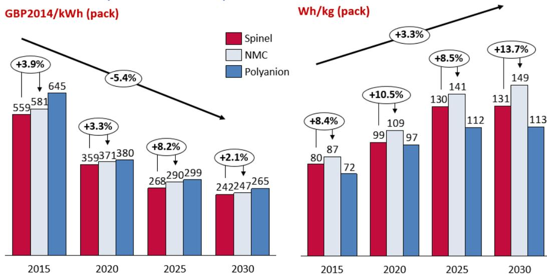
Figure 22 Cost and energy density projections for a 12 kWh PHEV battery pack (baseline scenario)
