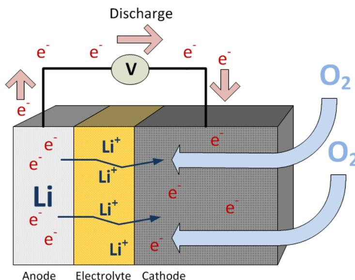
Figure 10. Lithium-air battery during a discharge cycle.
