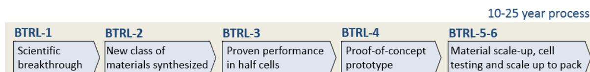
Figure 5. Battery Technology Readiness Level (BTRL) scale [6]
