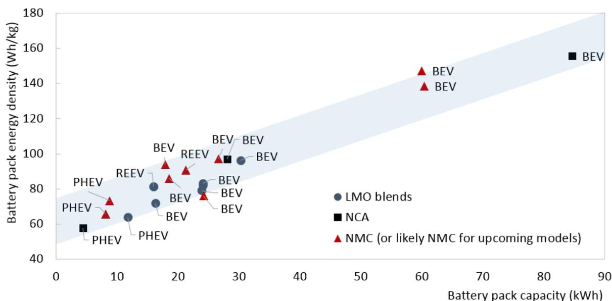
Figure 14 Relationship between battery pack energy density and the battery pack capacity for BEVs, REEVs and PHEVs <sup>27</sup>
