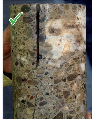
Figure 2.6 Compliant core, fine, full-depth vertical crack
