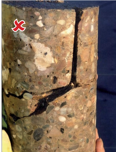
Figure 2.5 Non-compliant core, steel reinforcement not severed
