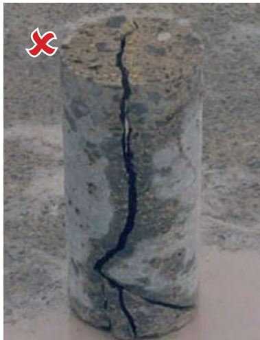
Figure 2.3 Non-compliant core, over-cracked
