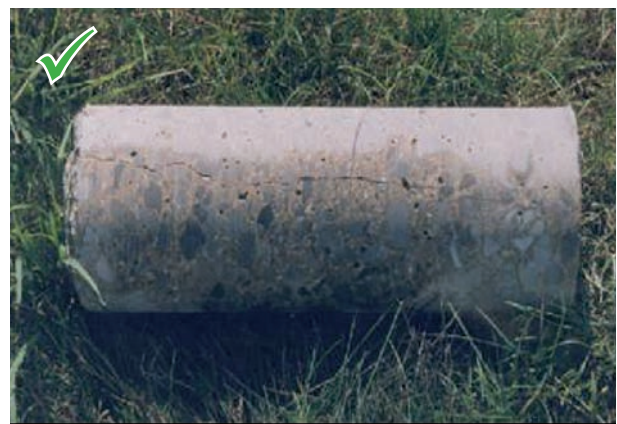
Figure 2.4 Compliant core, fine, full-depth vertical crack
