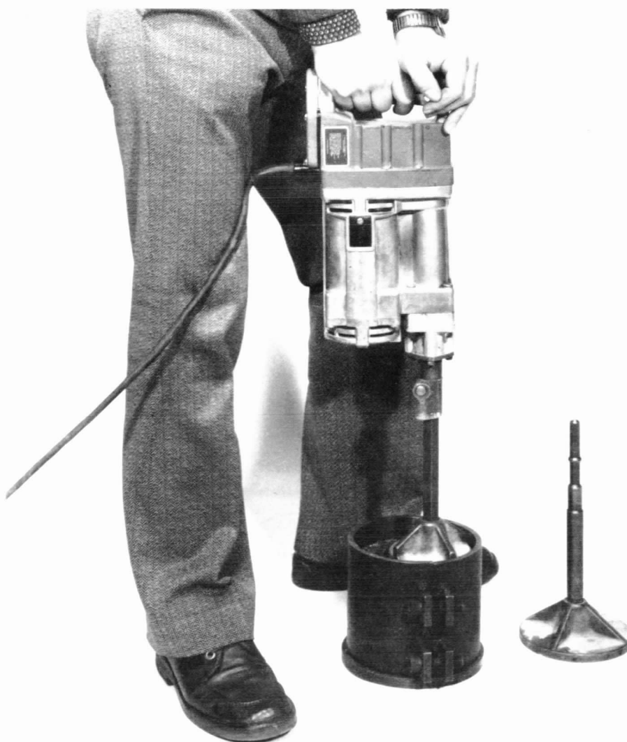
Plate 2 Sample in assembled mould at test temperature being compacted to refusal
