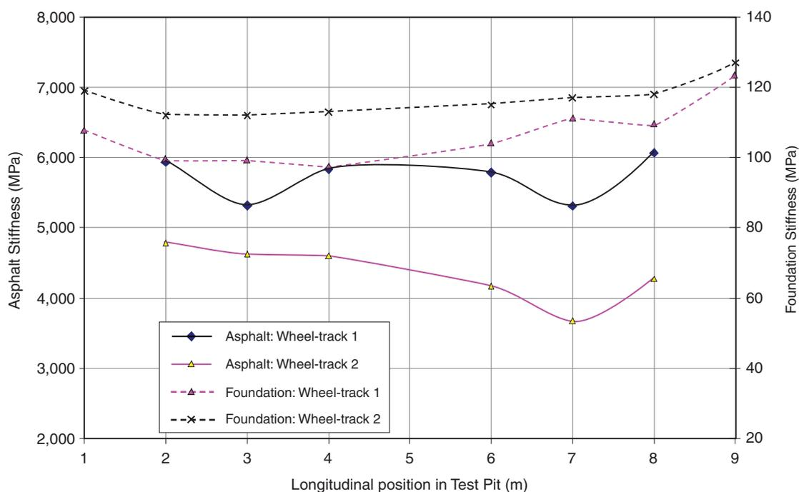
**Figure A.10** Stiffness of the bound layers and the foundation derived from FWD measurements
