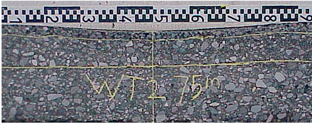
**Figure 8.10** Transverse section of wheel-track 2 at 7.5 m (EME Class 2 wheel-track inlay in HDM binder course)
