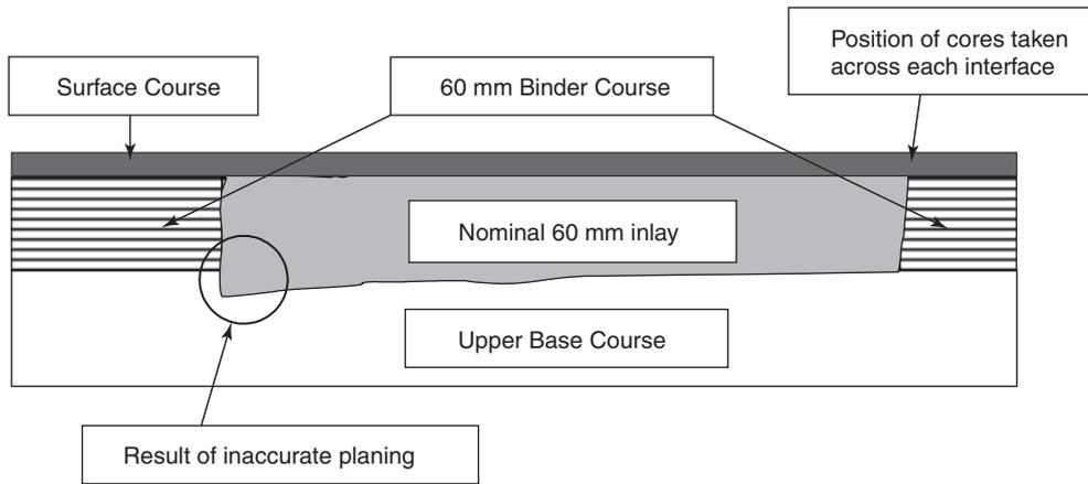
**Figure 8.11** Transverse section of wheel-track 2 after milling original binder course
