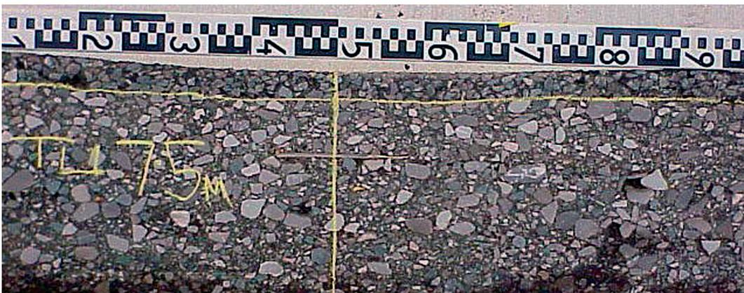
**Figure 8.9** Transverse section of wheel-track 1 at 7.5m (HDM full width inlay)
