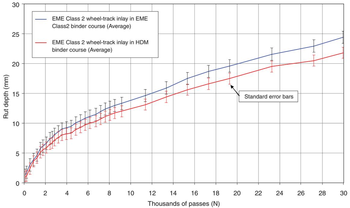
**Figure 8.4** Development of rut in wheel-track 2
