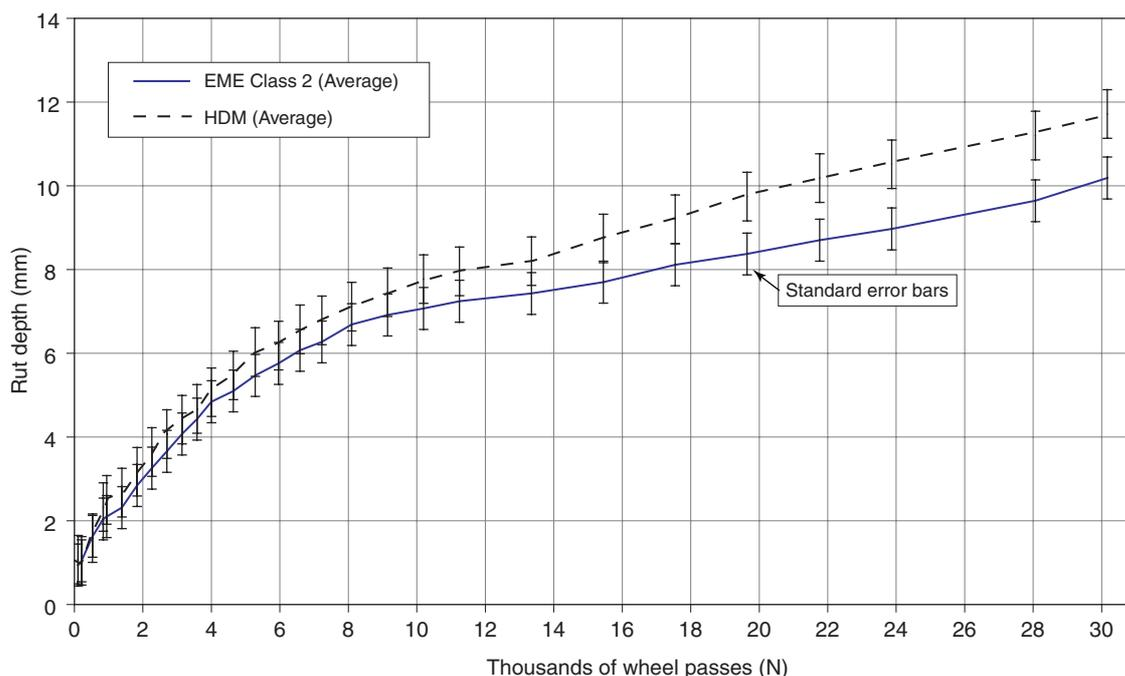
Figure 8.1 Development of rut in wheel-track 1
