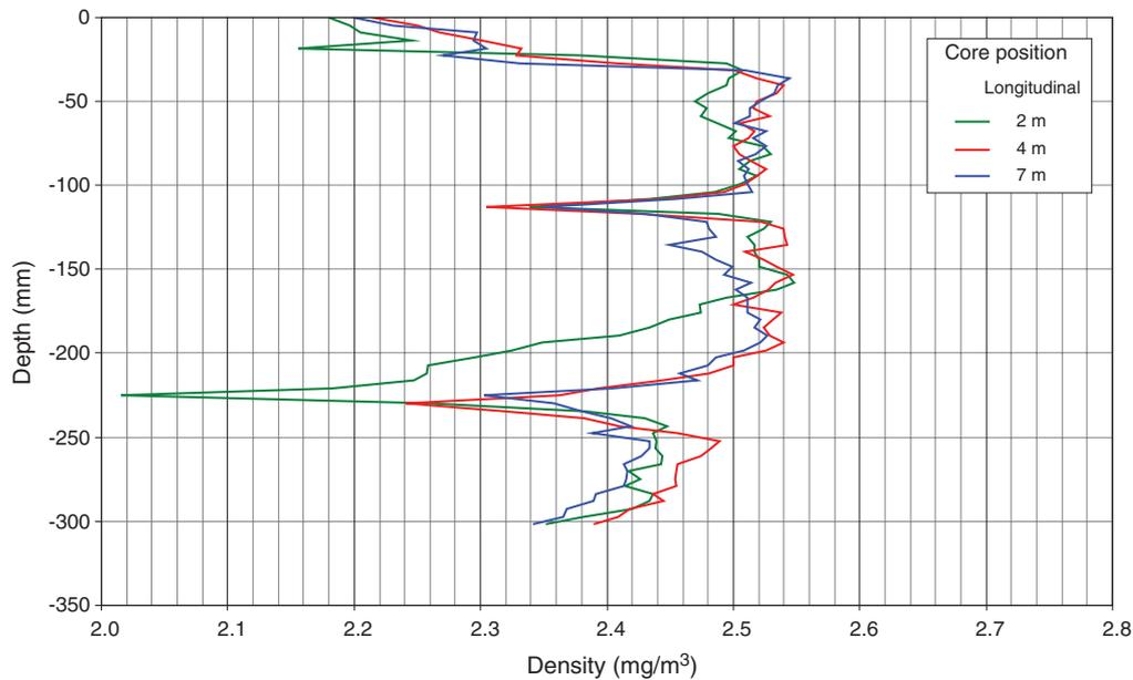
**Figure A.7** Density profile of cores from the untrafficked trench inlay of EME Class 2
