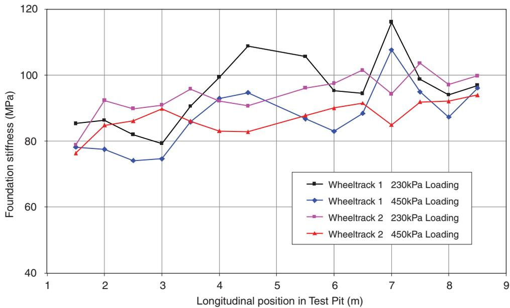
Figure A.3 PTF foundation stiffness derived from FWD deflections (before asphalt was placed)
