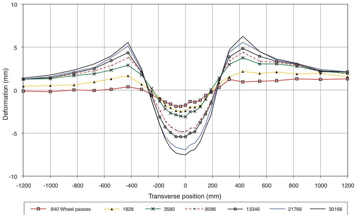
**Figure 8.3** Development of transverse profile in wheel-track 1 (full width inlay of HDM binder course)
