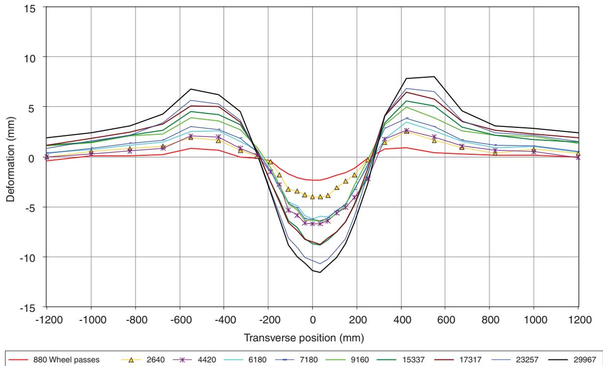
**Figure 8.6** Development of transverse profile in wheel-track 2 (EME Class 2 wheel-track inlay HDM binder course)
