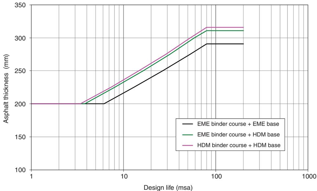
**Figure 10.2** A comparison of design curves for EME and HDM with Foundation Class 2
