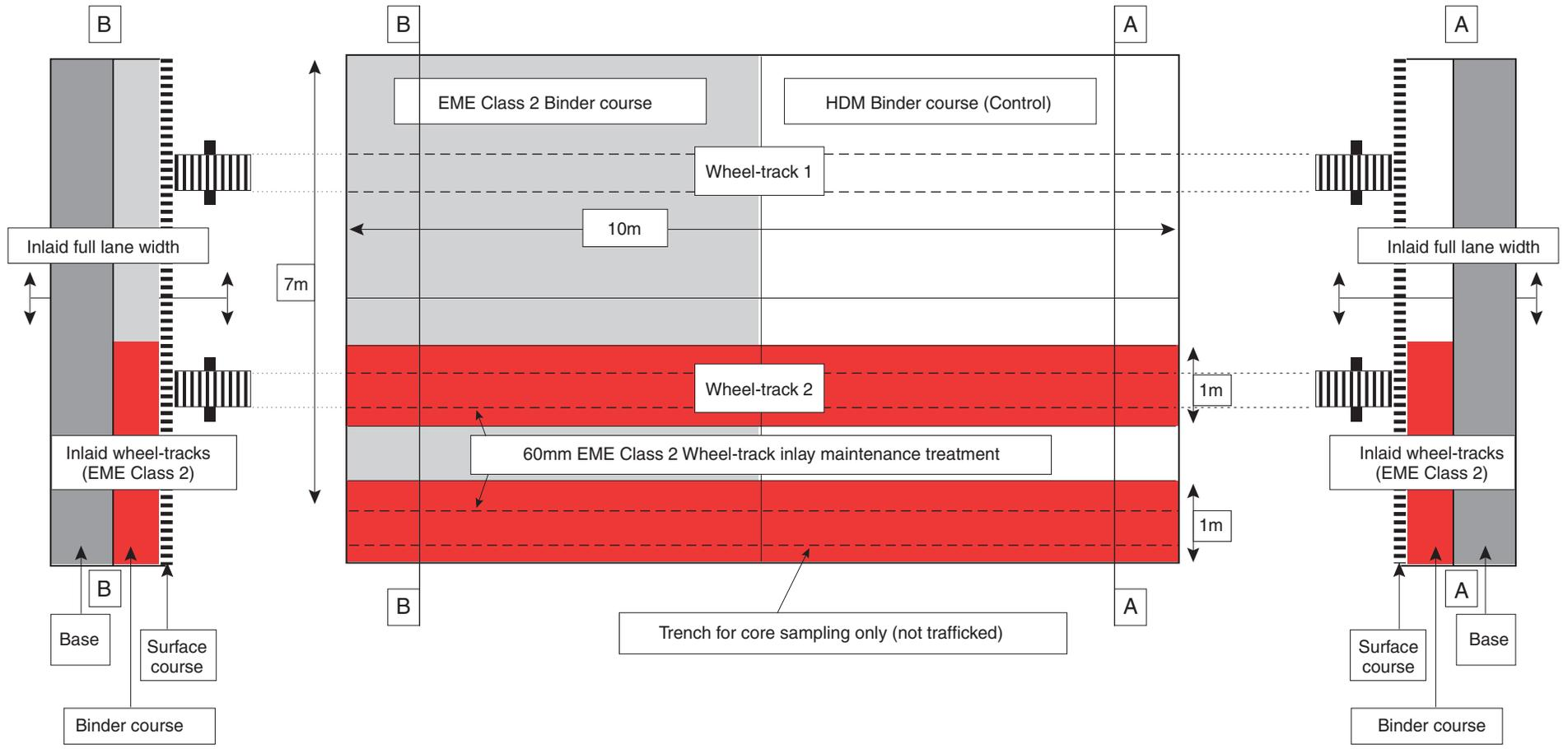
Figure 6.1 Plan and cross sections of test sections in the TRL pavement test facility
