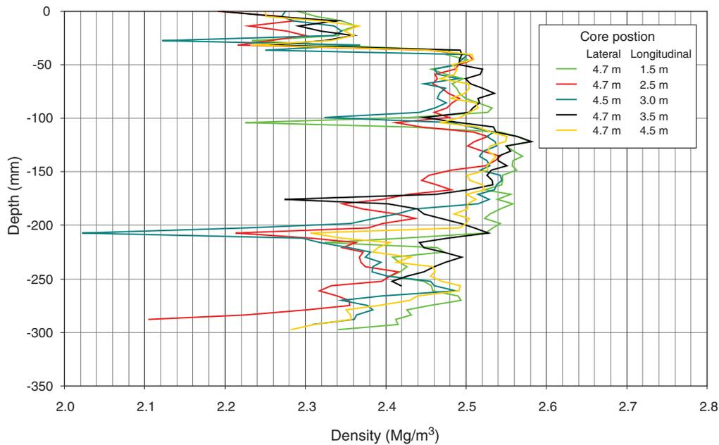
Figure A.5 Density profile of cores from the untrafficked EME Class 2 section
