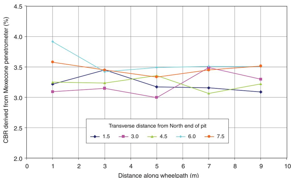
**Figure A.1** Subgrade strength from Mexecon penetrometer testing
