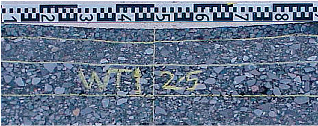
**Figure 8.7** Transverse section of wheel-track 1 at 2.5m (EME Class 2 full width inlay)
