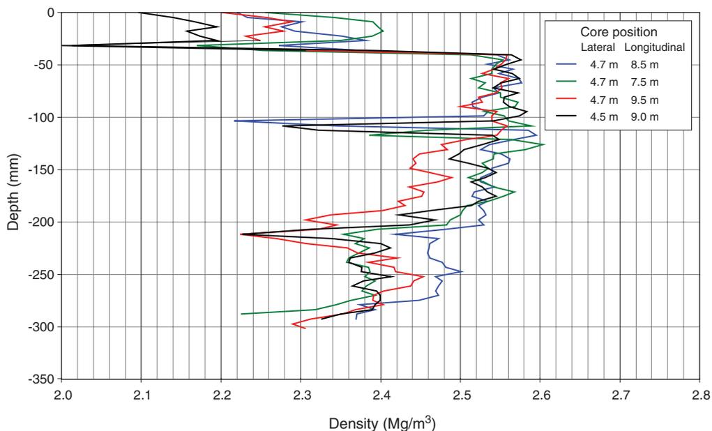
Figure A.6 Density profile of cores from the untrafficked HDM section
