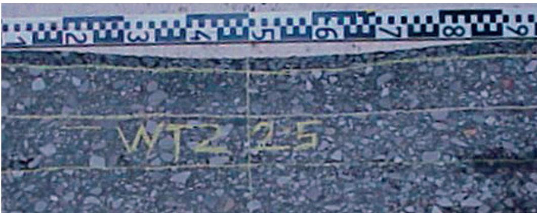
**Figure 8.8** Transverse section of wheel-track 2 at 2.5m (EME Class 2 wheel-track inlay in EME binder course)
