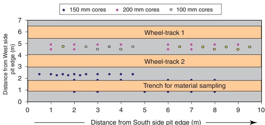
**Figure A.4 Core positions for material sampling**
