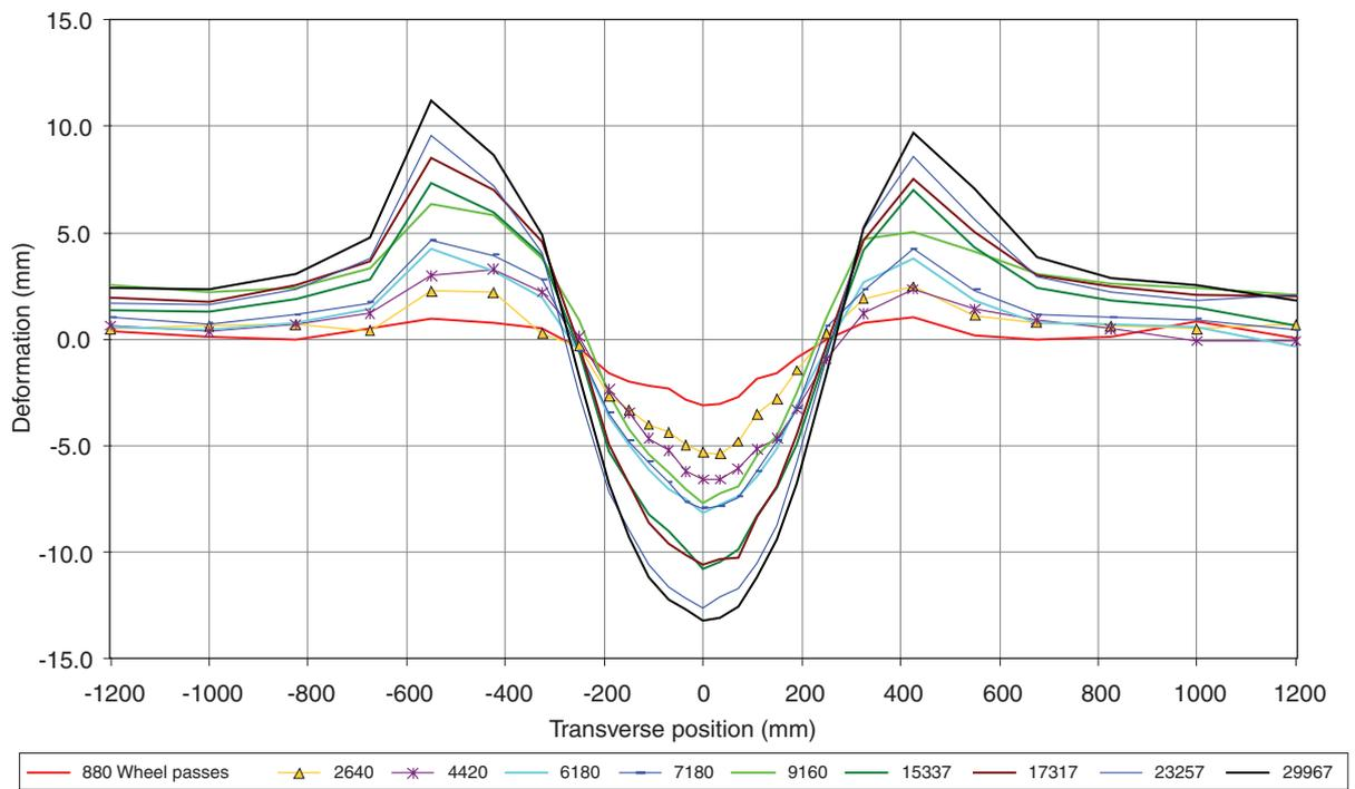
**Figure 8.5** Development of transverse profile in wheel-track 2 (EME Class 2 wheel-track inlay in EME Class 2 binder course)
