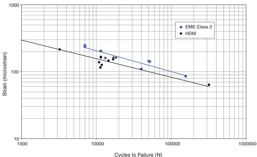
Figure 8.13 Comparison of ITFT fatigue behaviour of EME Class 2 and HDM
