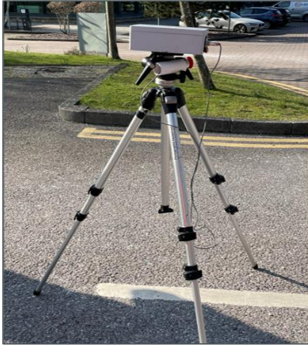
Figure 6: Speeds were measured using a radar speed gun mounted on a tripod at each end of the test area
