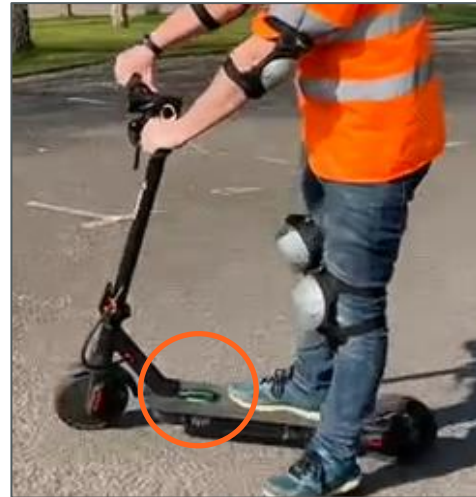
Figure 5: Device and rider with the accelerometer mounted on the footplate and rider standing centrally
