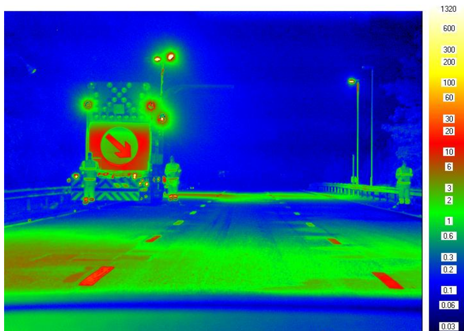
Figure 10-21: TTM/IPV scenario, luminance levels, additional lighting on
