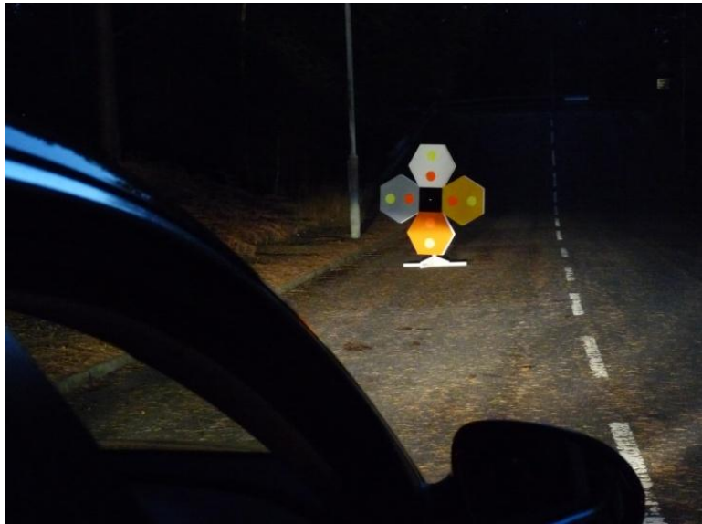
Figure 10-17: Colour board in place on test track (small road system) during night time trials
