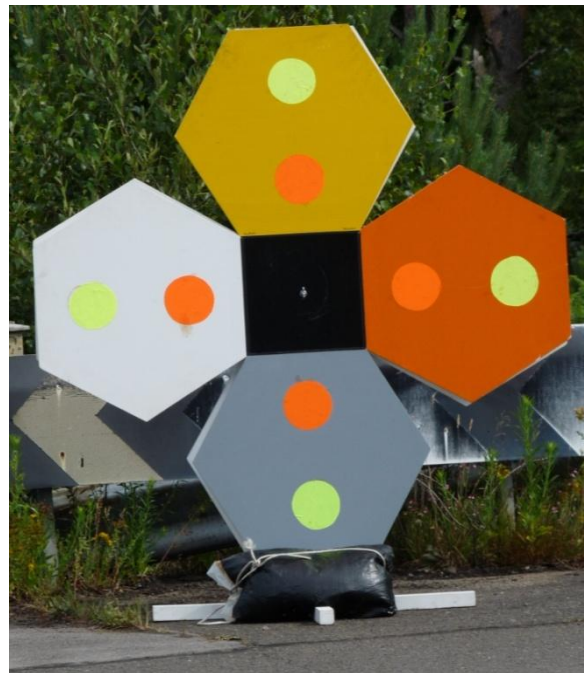
Figure 10-18: Colour board in place on test track during daytime trials
