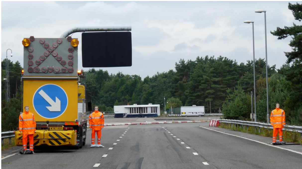
Figure 10-13: Road worker scenario, showing vehicle and mannequin positions
