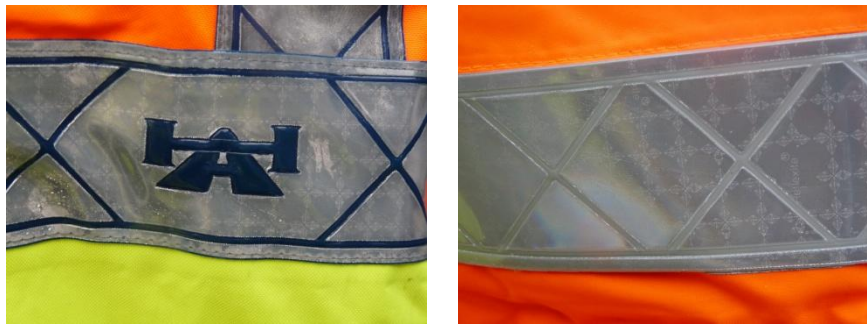
Figure 10-5: -specific retro-reflective tape (left), Reflexite GP440 (right)
