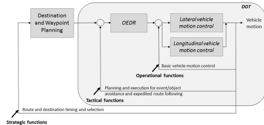
**Figure 1: Schematic view of driving task showing the dedicated driving task (DDT) portion. OEDR stands for Object and Event Detection and Response. Reproduced from (Society of Automotive Engineers, 2021).**
