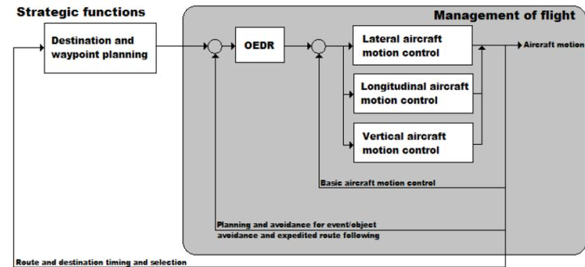
**Figure 4 Schematic of UAV Operation – schematic based on SAEJ3016, JUN2018 (reproduced from (European Cockpit Association, 2020))**
