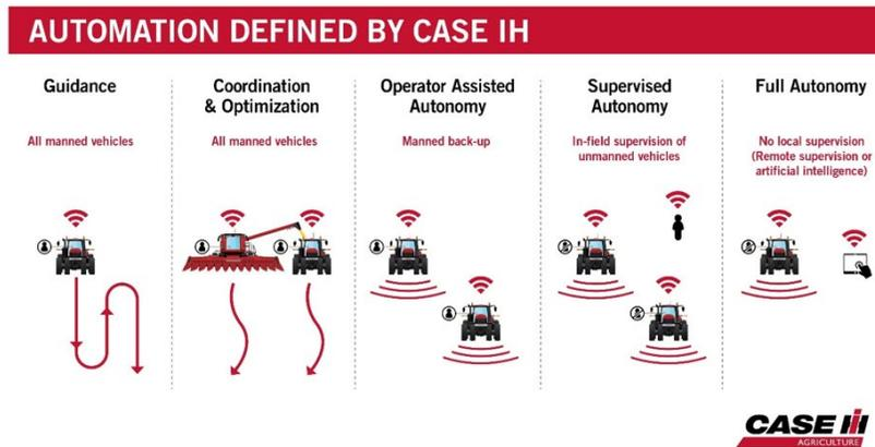
**Figure 2 Infographic showing 5 levels of automation proposed by Case IH, (Case IH, 2018)(Case IH, 2018)**
