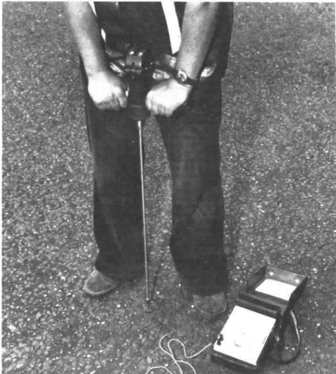
Plate 3 TRRL Probe Test for assessing road hardness (Inset: probe tip)
