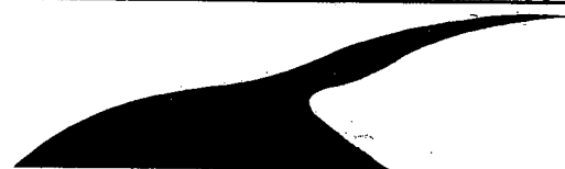
(d) A valley curve occurring within a horizontal curve
