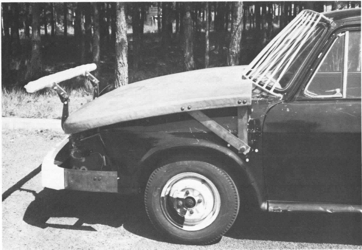
PLATE 4. Experimental front-end No. 2a with raised catcher device
