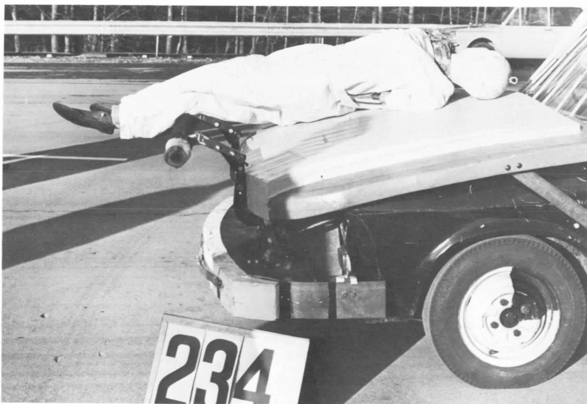
PLATE 6. Experimental front-end No. 2b retaining adult on bonnet at 16 km/h
