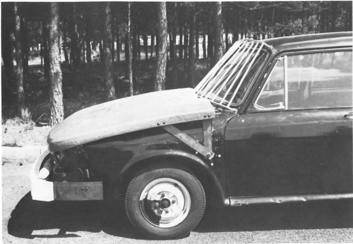
PLATE 3. Experimental front-end No. 2a with stowed catcher device
