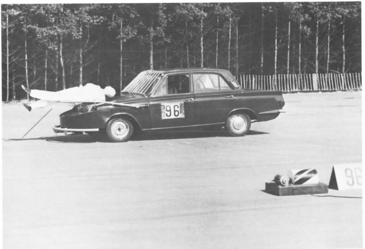
PLATE 2. Experimental front-end No. 1 retaining adult pedestrian
