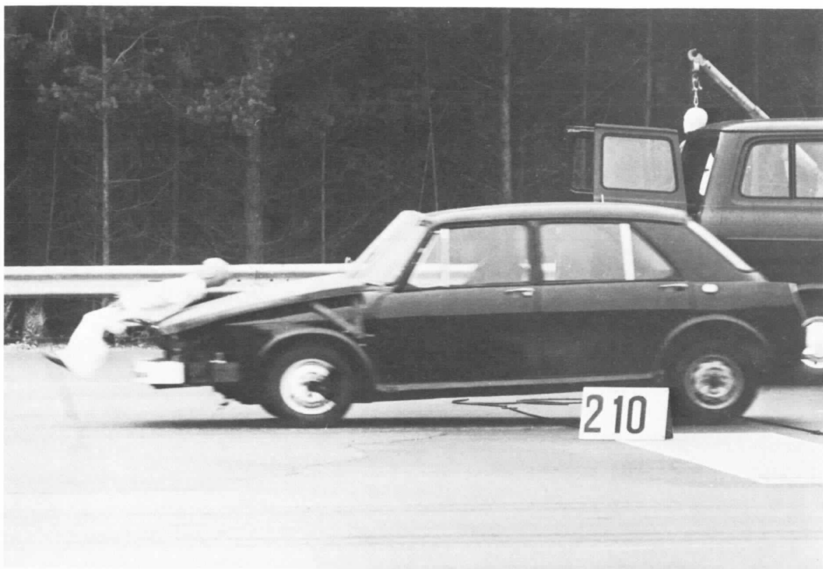
PLATE 5. Experimental front-end No. 2a picking up child at 16 km/h
