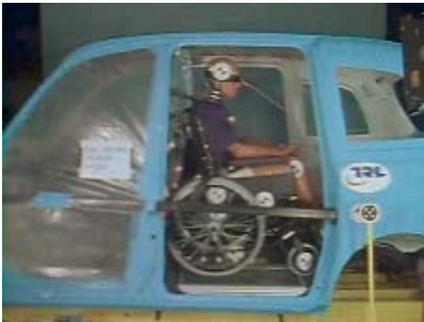
Figure 18a Set up with no head and back restraint
