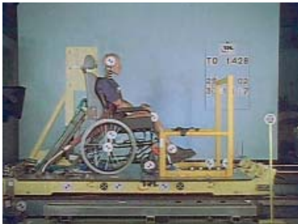
Figure 12a Set up with a head and back restraint
