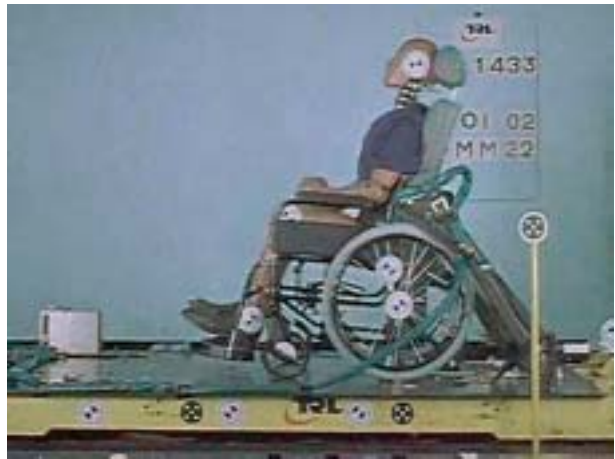
Figure 19b Wheelchair occupant with a head and back restraint
