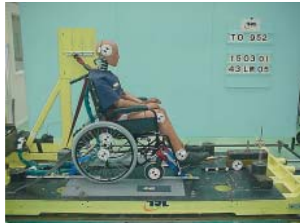
Figure 22 M3 forward facing wheelchair seated
