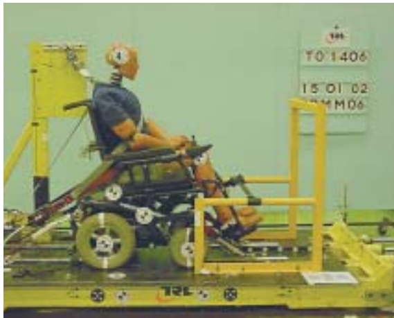
Figure 9 Set up with upper anchorage location for diagonal occupant restraint
