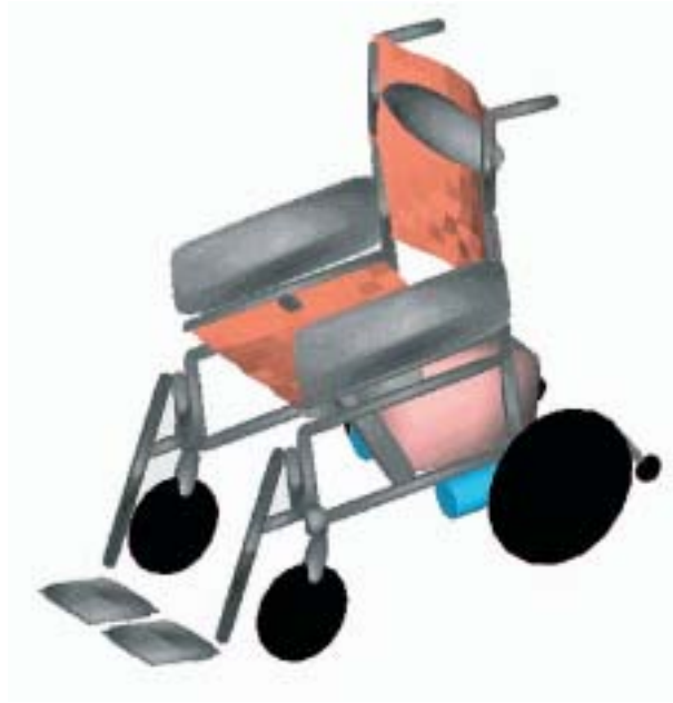
Figure C2 MADYMO model of the electric wheelchair
