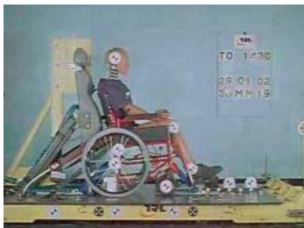
Figure 27a Set up with a gap between head and back restraint and occupant
