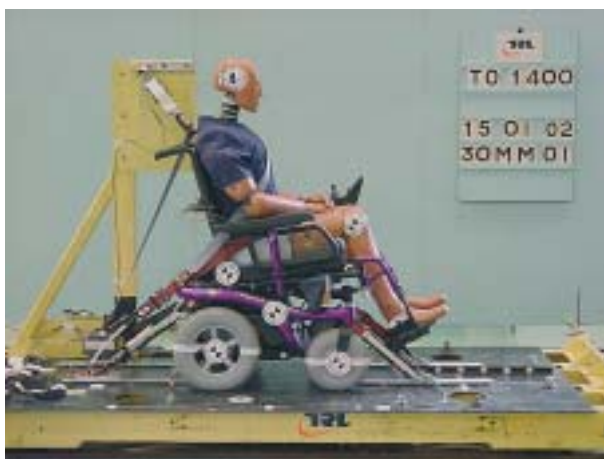
Figure 23 Set up with an upper location for the diagonal belt anchorage
