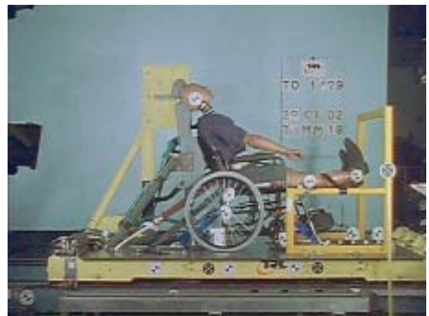
Figure 13b Wheelchair occupant with a gap between head and back restraint and occupant
