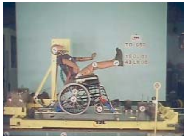
Figure 25b Wheelchair occupant with no head and back restraint
