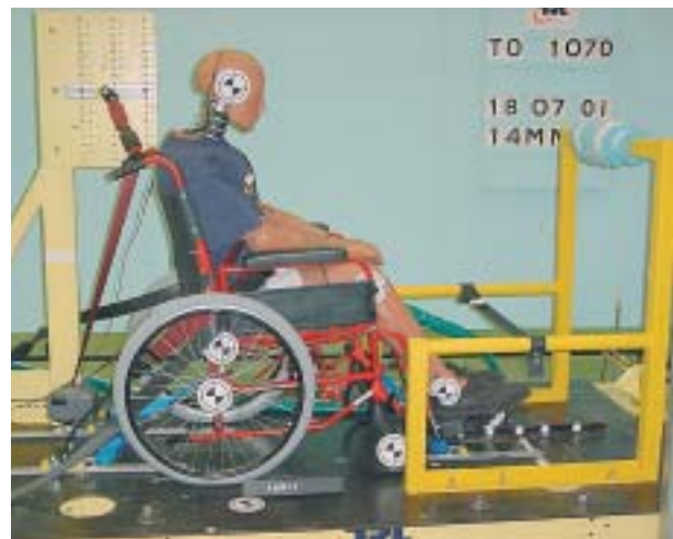
Figure 8 M1 and M2 forward facing – wheelchair seated
