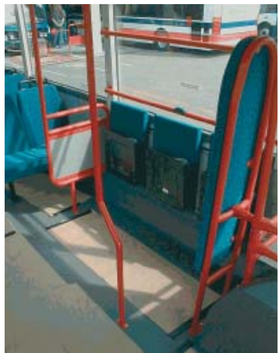
Figure 34 Wheelchair space in Optare Excel
