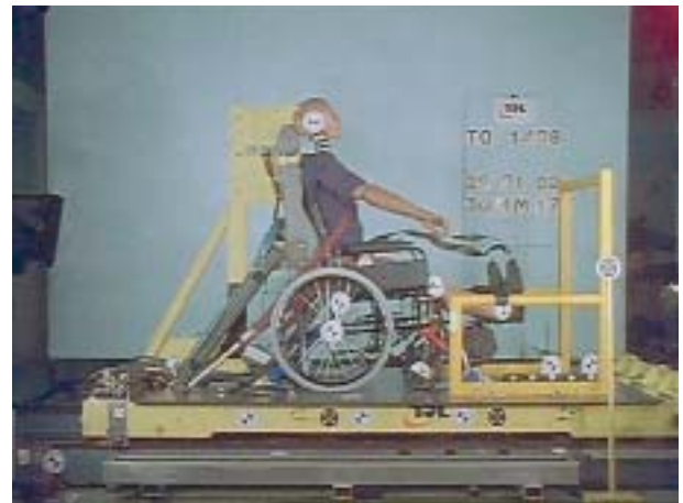
Figure 12b Wheelchair occupant with a head and back restraint
