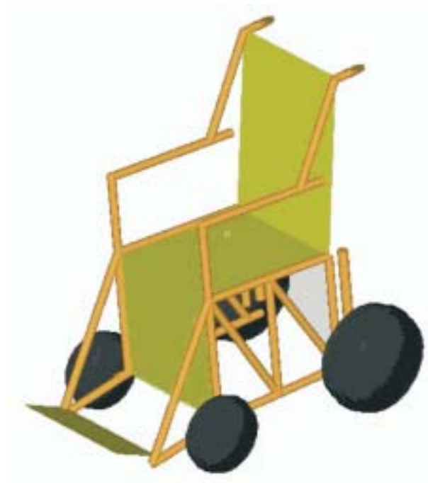
Figure C3 MADYMO model of the surrogate wheelchair
