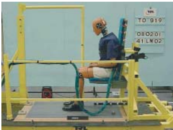
Figure 29 M3 rear facing – vehicle seated
