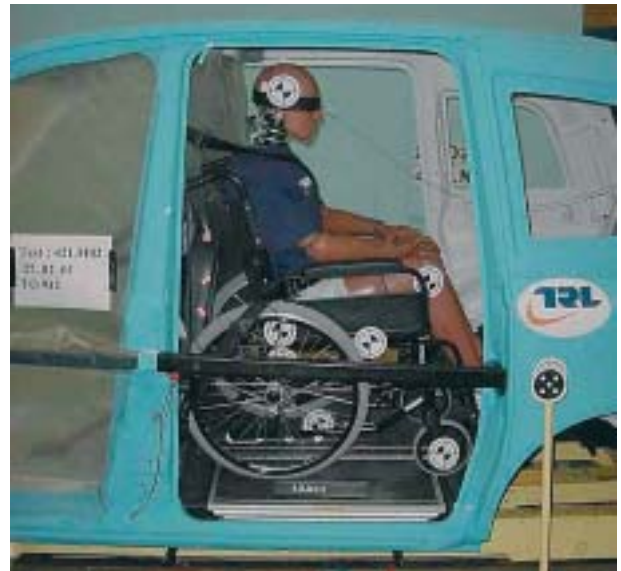
Figure 16 M1 and M2 rear facing – wheelchair seated
