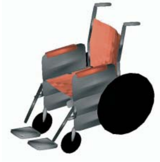
Figure C1 MADYMO model of the manual wheelchair
