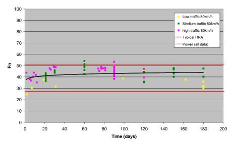
Figure 8.8 Change in wet friction at 80km/h over time for surfacings from 0-6 months old
