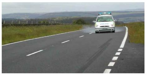
Figure 4.3 Police car conducting a "Skidman" dry test
