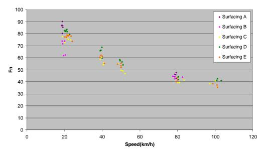
Figure 8.1 Illustration of the scatter in replicate wet friction measurements using the PFT at different speeds on five different surfaces of similar age
