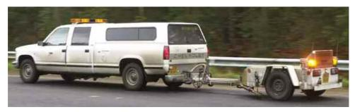
Figure 4.2 The Pavement Friction Tester
