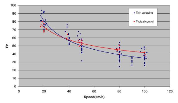
Figure 8.3 Wet friction measurements at different speeds on all sites from 1 day to 18 months old
