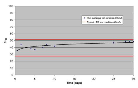
Figure 8.11 Development of higher-speed wet friction in the first month on the M3 sites
