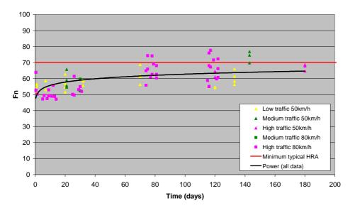
Figure 8.14 Change in dry friction at 50 or 80km/h over time for surfacings from 0 - 6 months old
