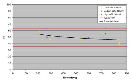
Figure 8.9 Change in wet friction at 50km/h over time for surfacings from 6-18 months old
