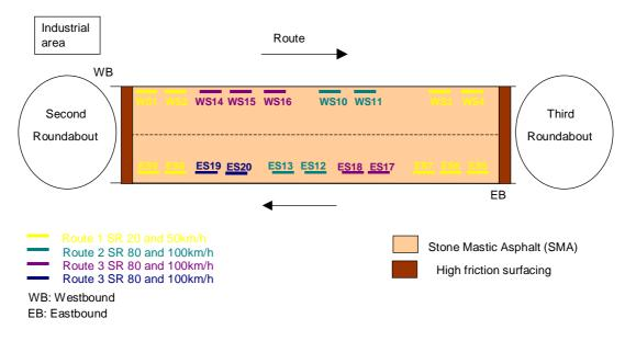
Figure A2: Schematic plan, western section, A511
