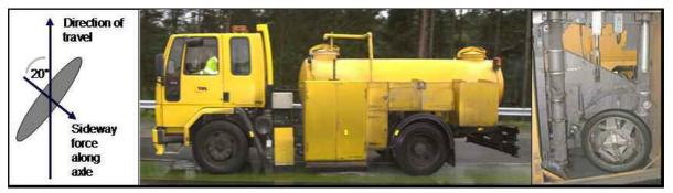
Figure 4.1 SCRIM – principle and test wheel detail
