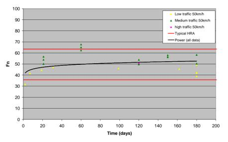
Figure 8.7 Change in wet friction at 50km/h over time for surfacings from 0-6 months old
