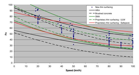
Figure 8.4 Comparison of wet friction and speed for new thin surfacings with typical ranges for different types of well-trafficked surfacing
