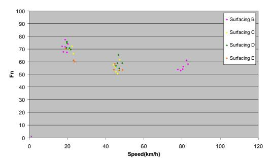
Figure 8.2 Illustration of the scatter in replicate dry friction measurements using the PFT at different speeds on four different surfaces of similar age
