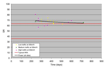
Figure 8.6 Change in low-speed wet skid resistance (SR) over time for surfacings from 6-18 months old
