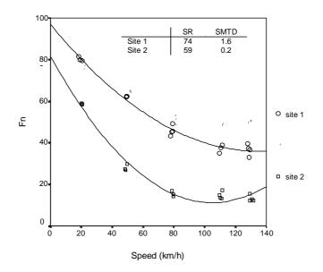
Figure 9.1: Wet friction versus speed two different "normal" surfaces
