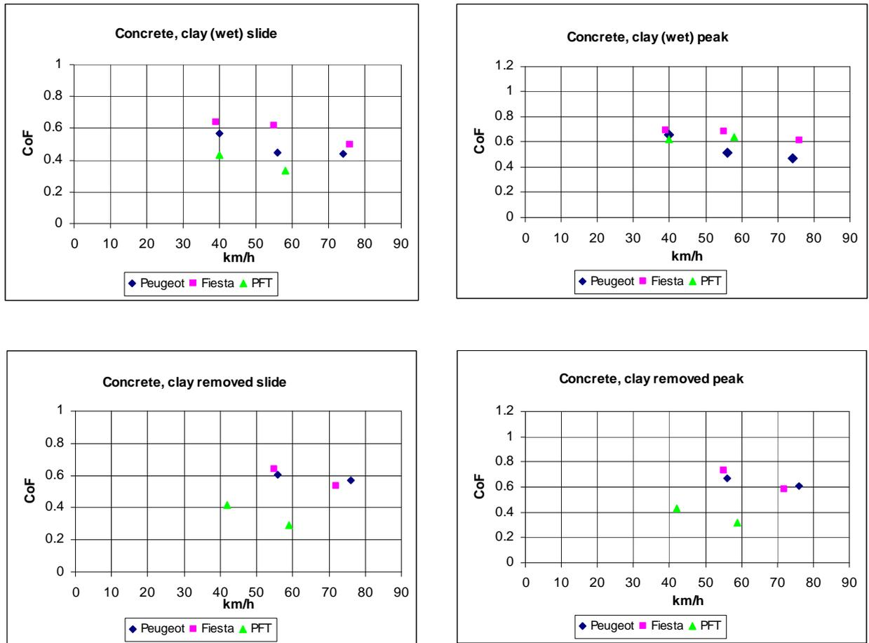
Figure 4.14 Coefficients of friction on concrete covered with wet clay
