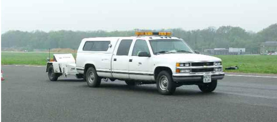
**Figure A1 KJ Law Pavement Friction Tester on the Asphalt Surface**
