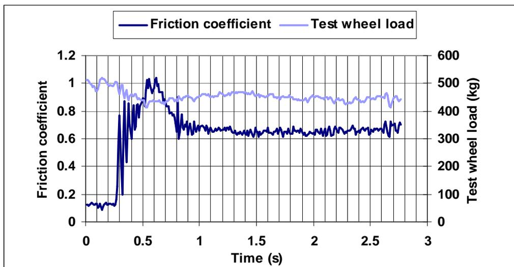
Figure 4.3 PFT graph for 60km/h test on wet asphalt
