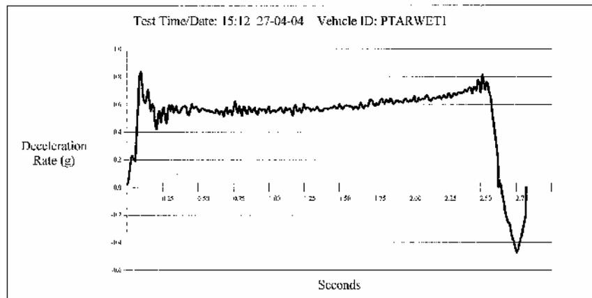
Figure 4.2 SkidMan graph for Peugeot sliding to a halt from 60 km/h on wet asphalt
