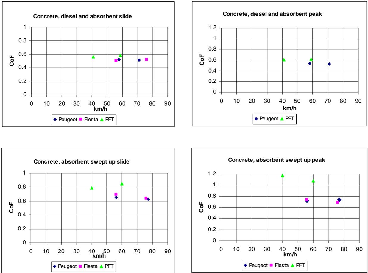
**Figure 4.10 Coefficients of friction on concrete covered with diesel fuel and absorbent**
