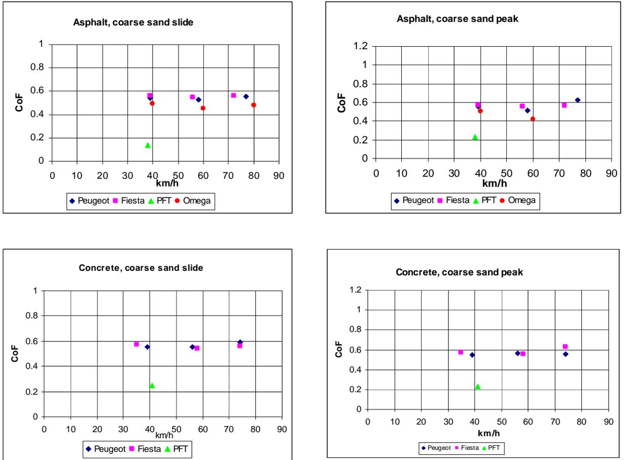
Figure 4.15 Coefficients of friction on asphalt and concrete covered with coarse sand
