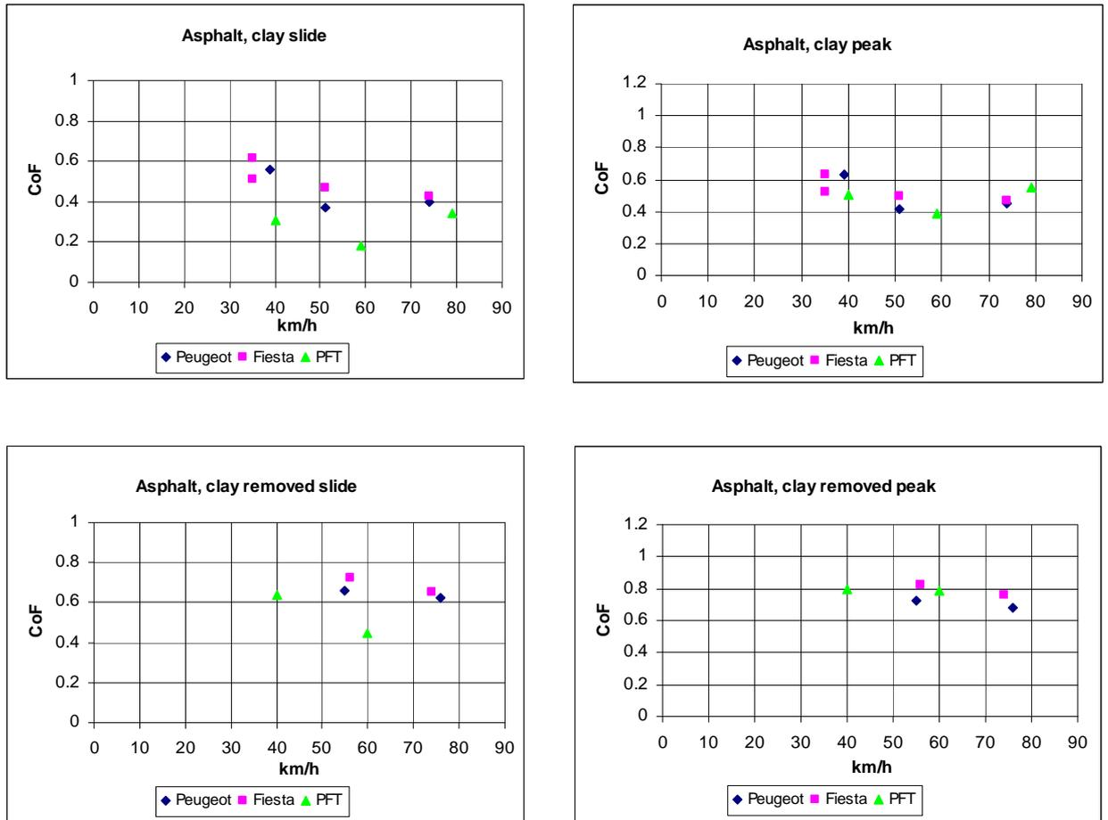
Figure 4.11 Coefficients of friction on asphalt covered with wet clay
