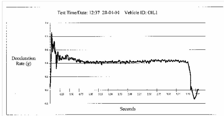
Figure 4.5 SkidMan graph for Fiesta sliding to a halt from 60 km/h on asphalt contaminated with waste engine oil
