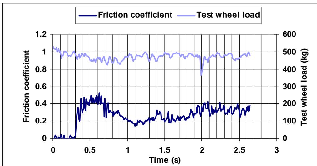
Figure 4.9 PFT graph for 60km/h test on concrete contaminated with diesel
