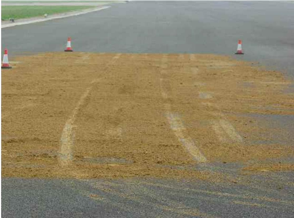
**Figure A7 Coarse sand on Asphalt (with braking marks from skid cars)**
