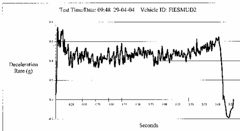
Figure 4.12 SkidMan graph for Fiesta sliding to a halt from 60 km/h on asphalt covered with wet clay
