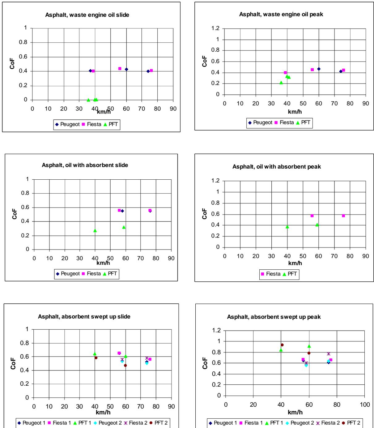
**Figure 4.4 Coefficients of friction on asphalt with waste engine oil**
