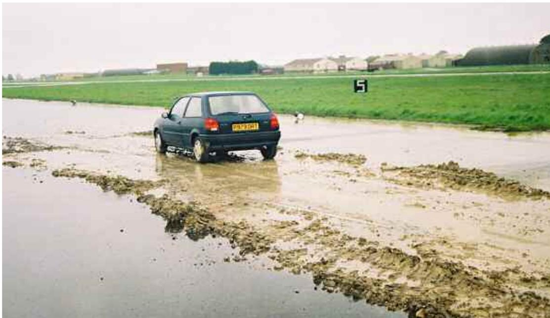
**Figure A6 Clay on Asphalt, with Ford skid car**
