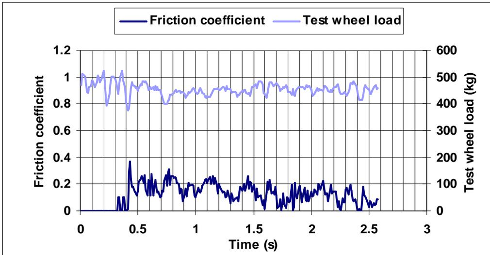
Figure 4.17 PFT graph for 60km/h test on asphalt contaminated with sand
