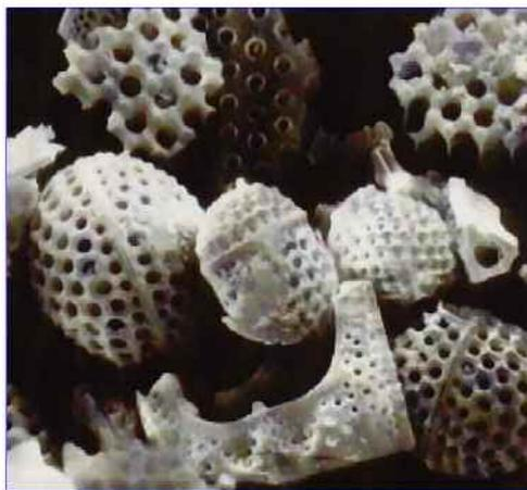
**Figure A4 Photomicrograph of Steetley Diatomaceous Earth**
