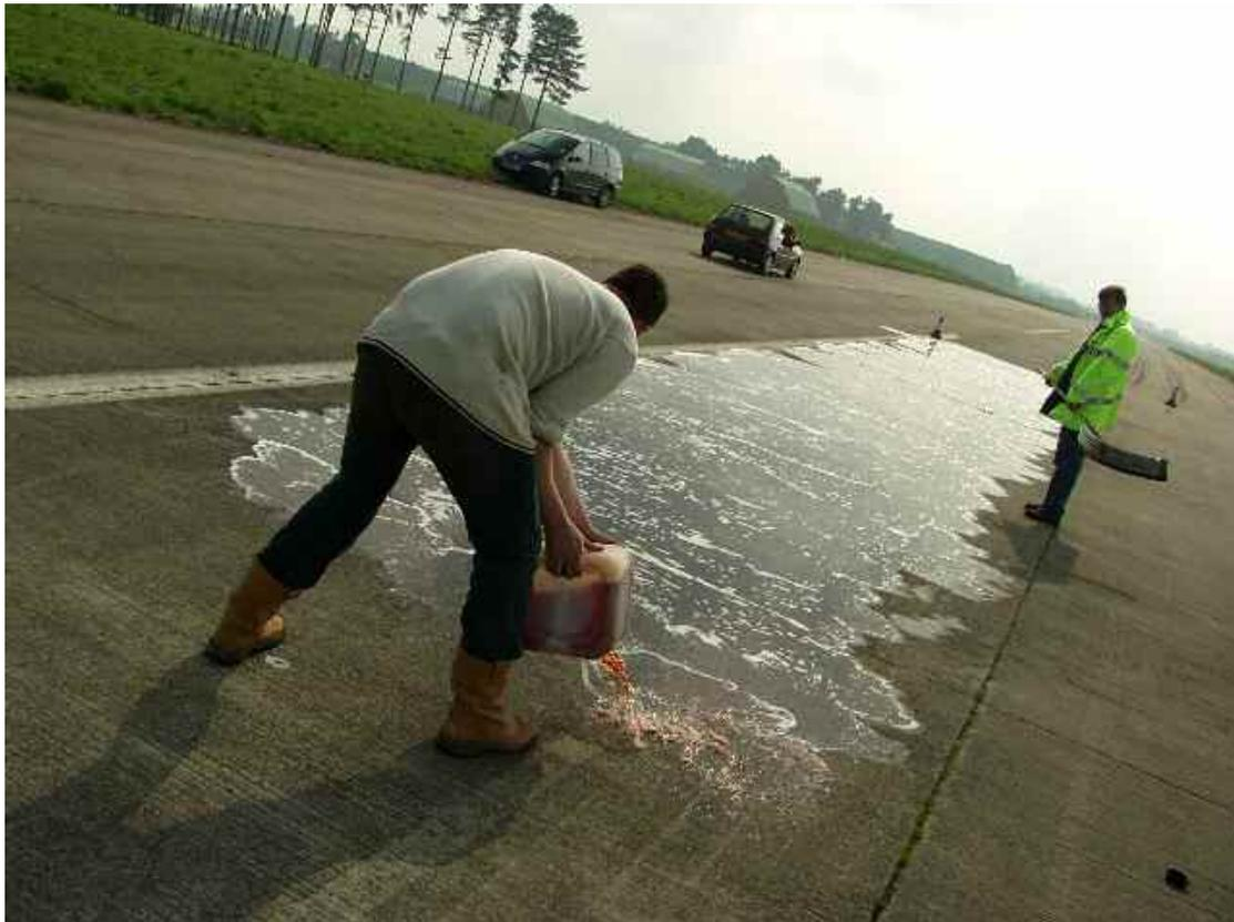
**Figure A3 Diesel Oil being spread on Concrete**
