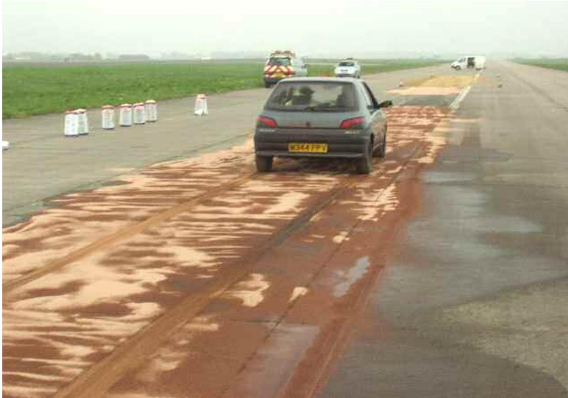
**Figure A5 Absorbent spread over engine oil, together with Peugeot skid car**
