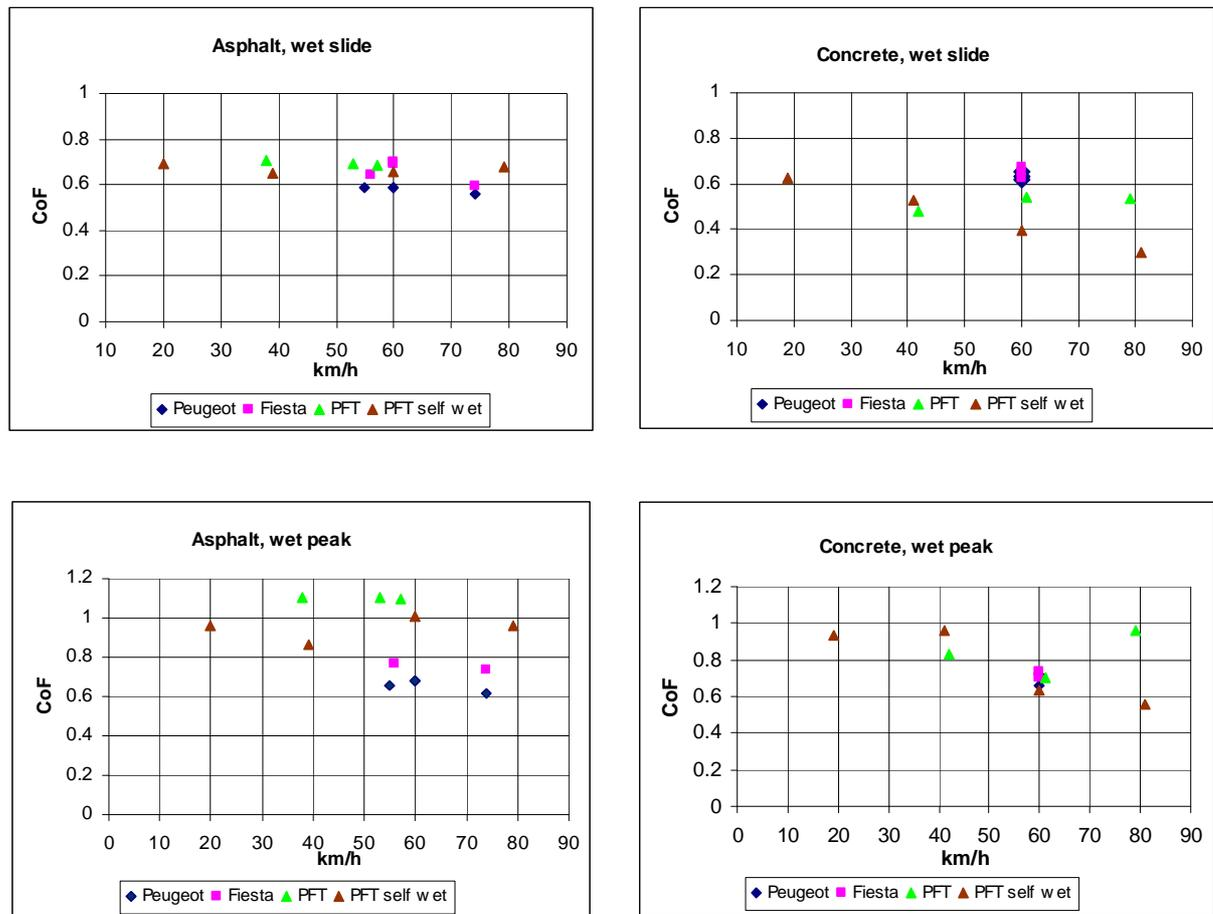
**Figure 4.1 Coefficients of friction on wet asphalt**
