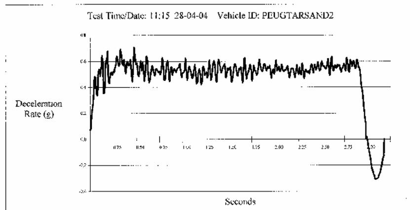
Figure 4.16 SkidMan graph for Peugeot sliding to a halt from 60 km/h on asphalt covered with coarse sand
