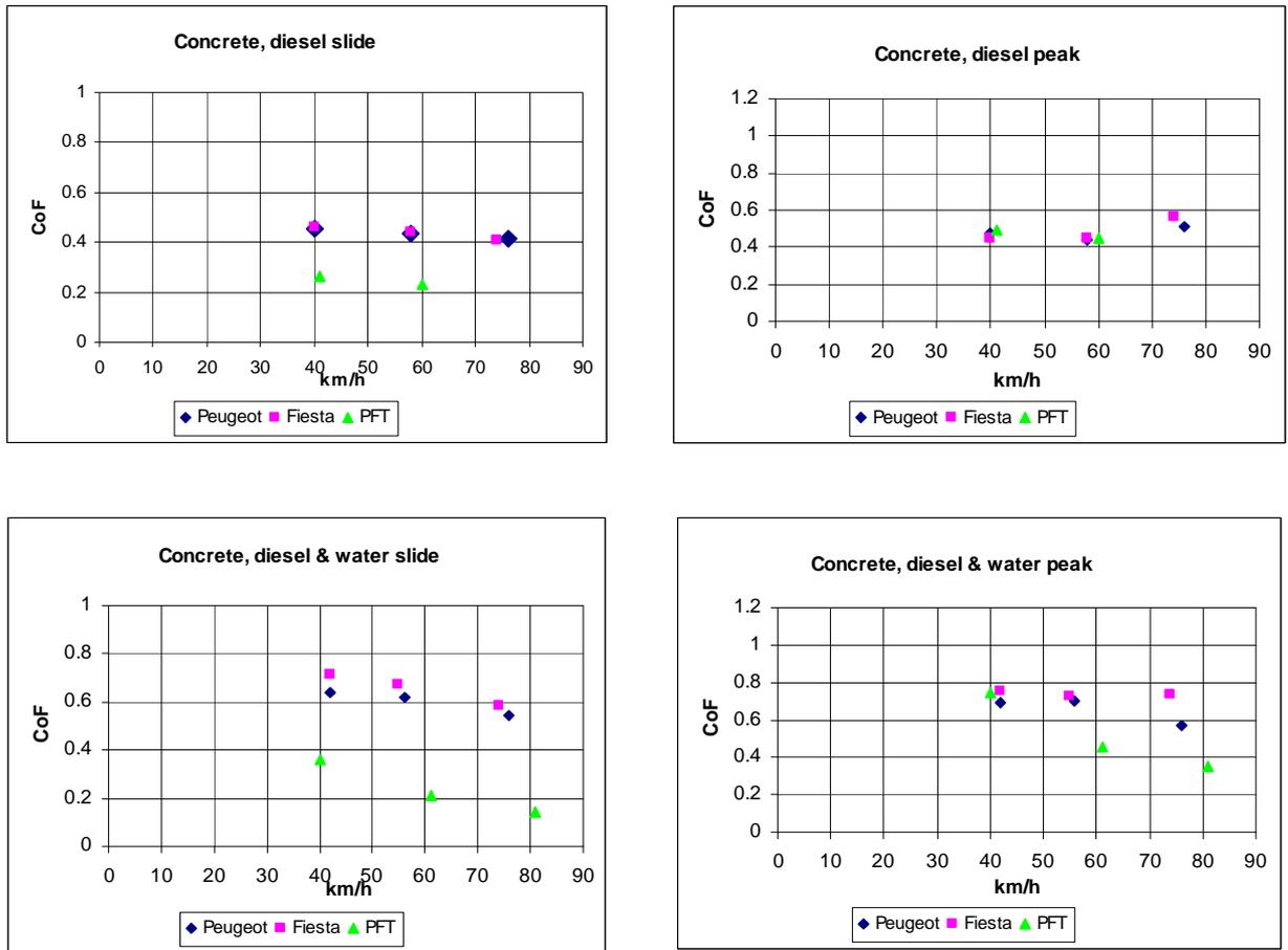
**Figure 4.7 Coefficients of friction on concrete covered with diesel fuel**
