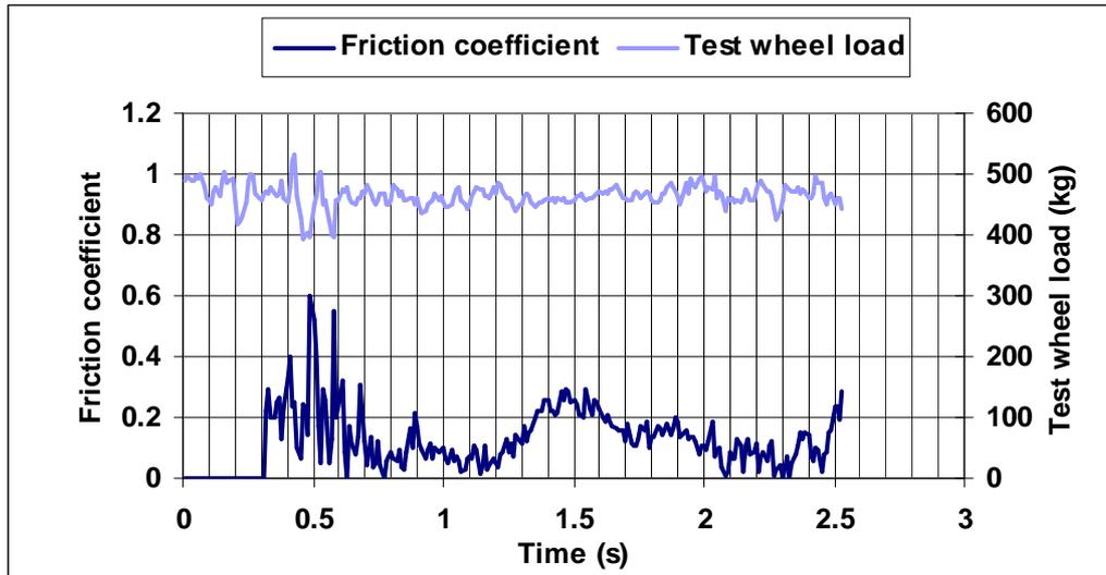
Figure 4.13 PFT graph for 60km/h test on asphalt contaminated with clay
