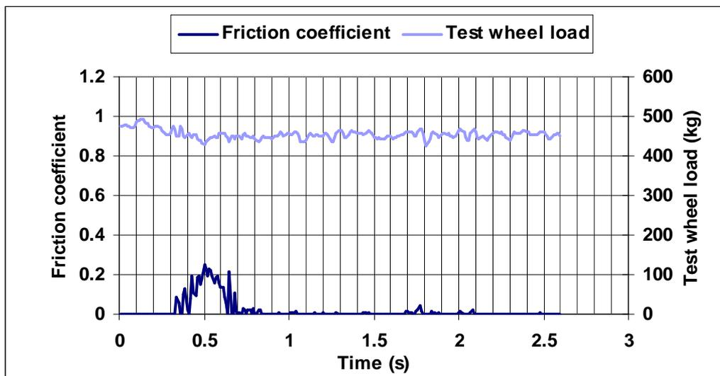
Figure 4.6 PFT graph for 35km/h test on asphalt contaminated with waste engine oil
