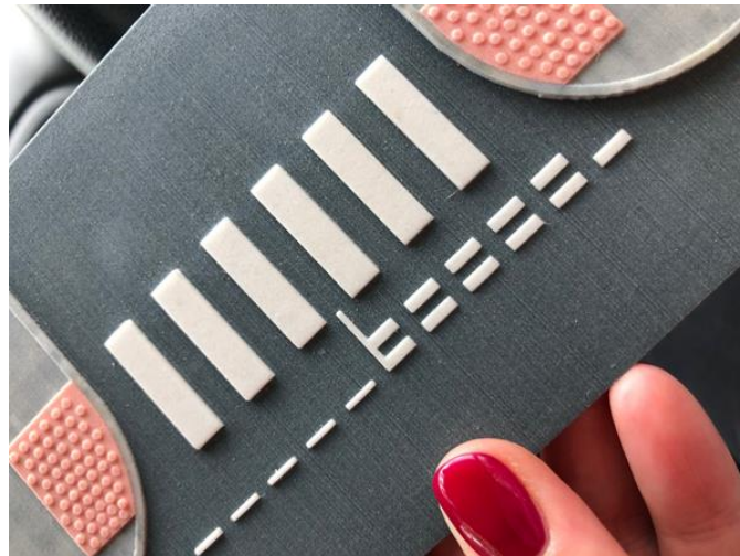
Figure 12: 3D Tactile model of non-prescribed zebra crossing sent to blind or visually impaired participants (with finger reference showing scale)
