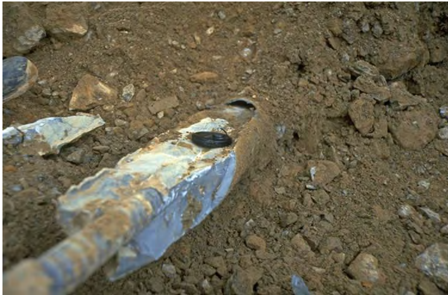
Figure 3.19: Construction of the A74 (M74 Junction 14 to 15) Tinny Bank soil nails trial in 1994/5; the beginning of a grout bulb can be seen in the partially excavated soil nail (cavitation of the grout annulus is also evident) (image the authors)
