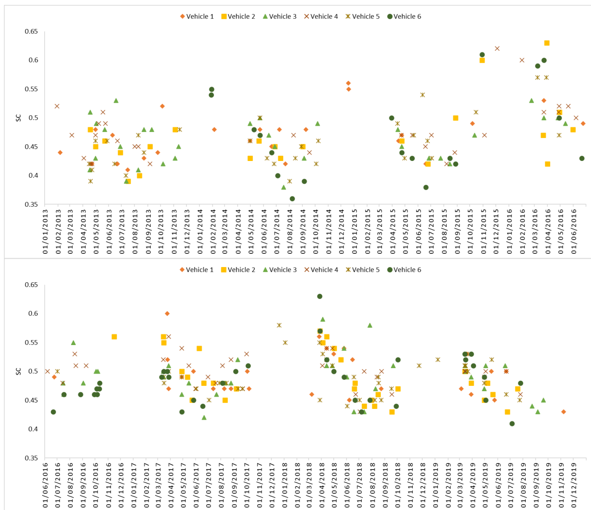
Figure 9: SC variation for sideways-force devices on the Bristol site over the period 2013-2019
