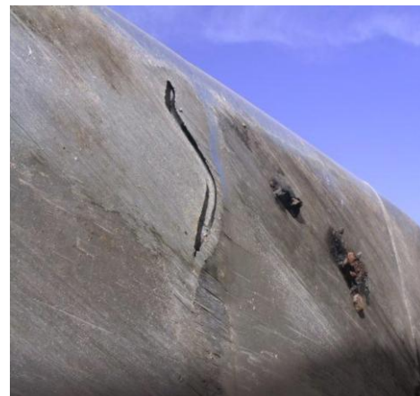
Figure 3-1: Offside view of damage to tank as a result of 90 degree roll and slide to rest (left) and close up of hole in tank showing signs of abrasion (right)
