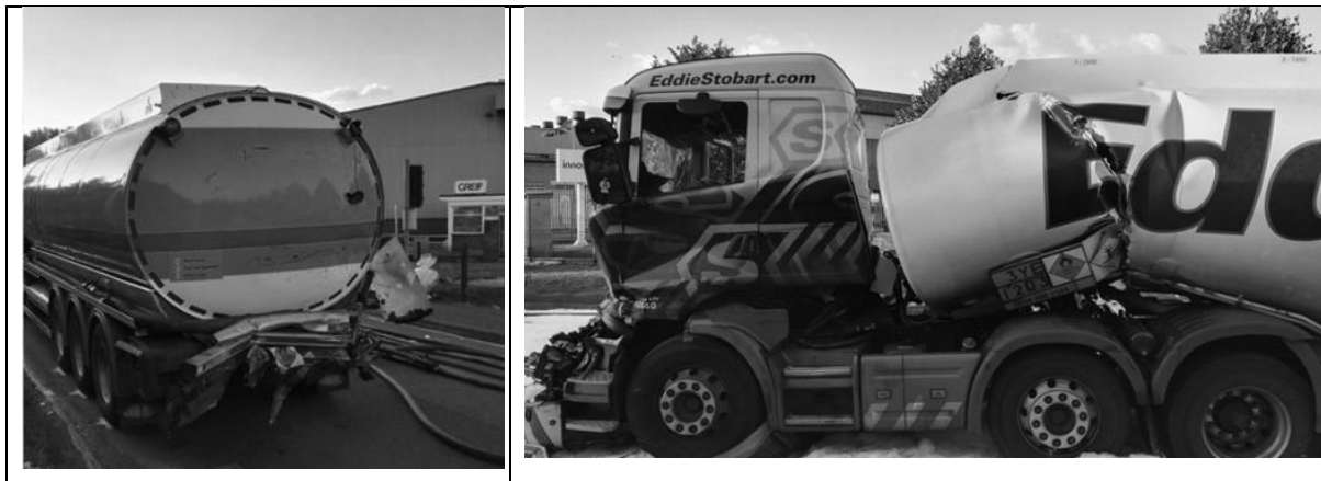
Figure 2-1: Pictures of baseline collision showing minimal deformation of tank of struck tanker and failure of striking tanker tank just behind the king pin
