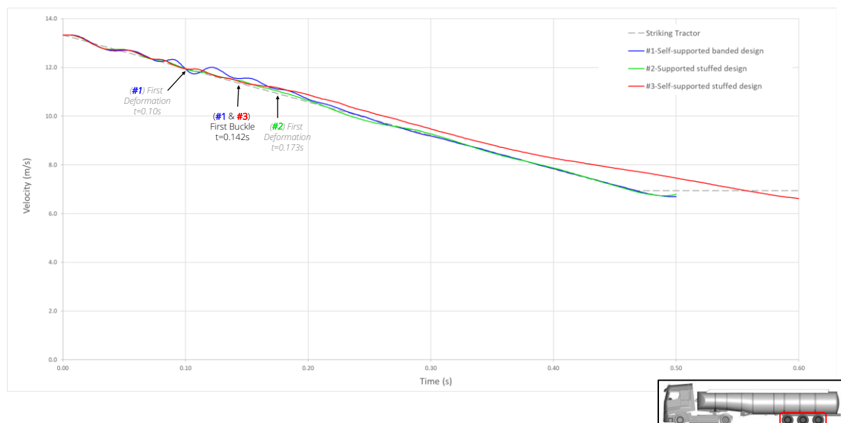
Figure 2-34: Comparison of semi-trailer rear (axle) velocities for 1.4 g fixed king pin deceleration parameter sweep. Note that dashed grey line represents the deceleration boundary condition constraint applied to the king pin
