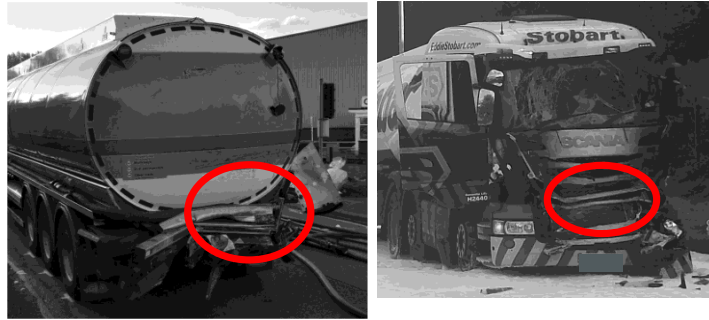
Figure 2-20: Identification of load path 2 between striking tanker cab/engine and struck tanker chassis rails
