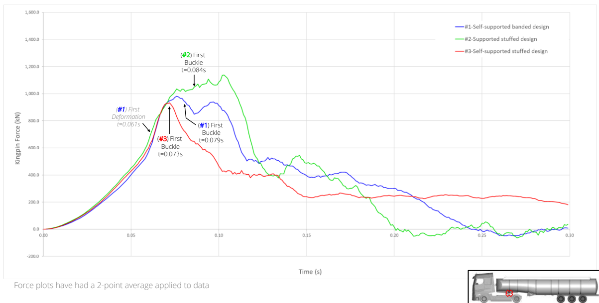
Figure B.2: Comparison of semi-trailer king pin force in longitudinal (x) direction for striking tanker at 18 km/h
