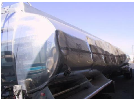
Figure 3-1: Offside view of damage to tank as a result of 90 degree roll and slide to rest (left) and close up of hole in tank showing signs of abrasion (right)
