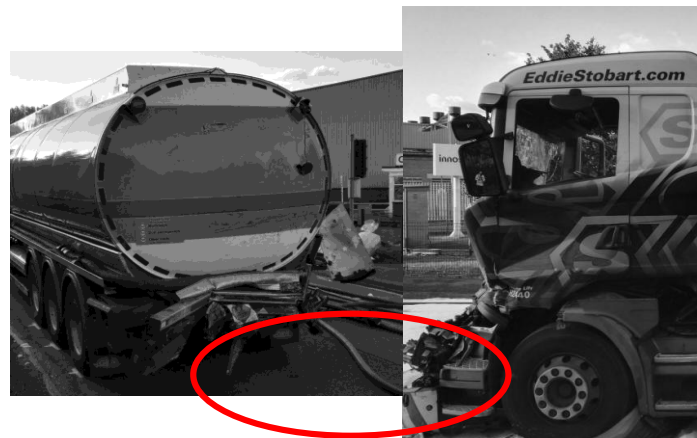
Figure 2-19: Identification of load path 1 between striking tanker chassis rails and struck tanker underrun guard
