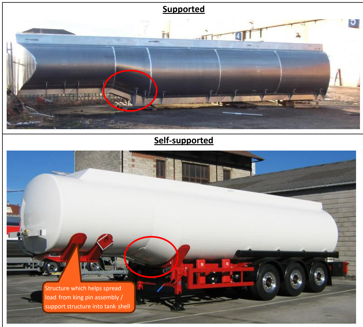
Figure 2-12: Examples of semi-trailer tanker designs which are supported and self-supported in the region of the conical / taper section behind the king pin assembly / support structure (indicated with red circle)
