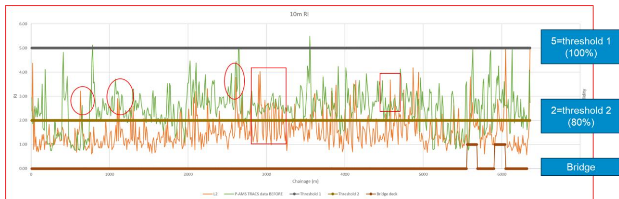
Figure 13 Example of where spikes in RI either remained after resurfacing or were introduced as a result of the works
