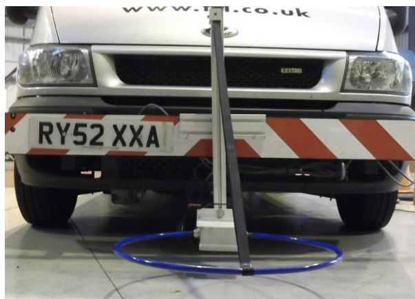
Figure 5-1 60cm antenna mounted on HARRIS2
