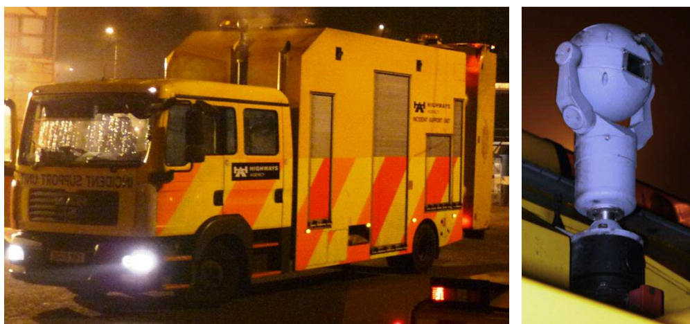
Figure 68: Incident Support Unit, with CCTV camera mast installed behind the cab
