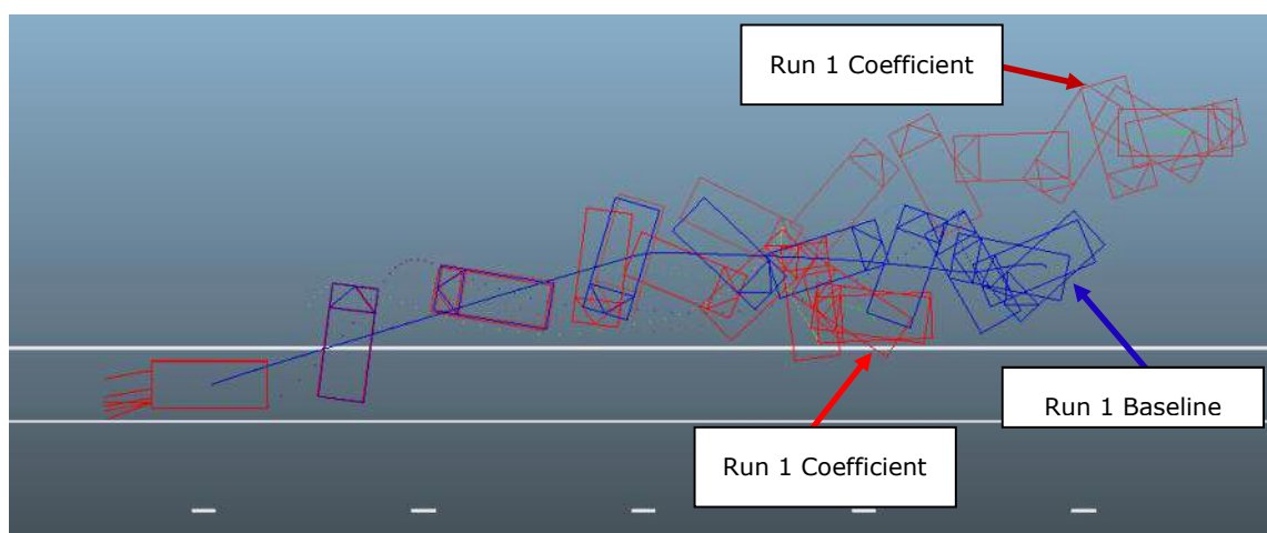
Figure 37: The track and displacement of the TOV in the HVE Simulation in Run 1 showing the effect of a change in coefficient of friction between the tyres and the road surface
