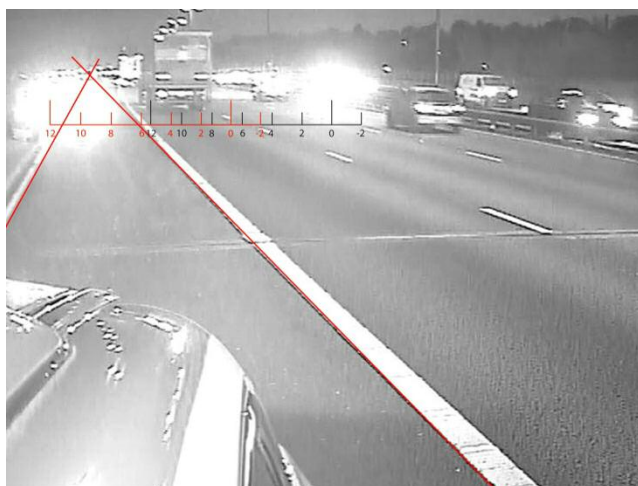
Figure 11: Identifying fender angle from incident video
