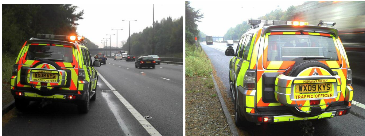
Figure 54: TOV parked in fend off orientation; note proximity of front offside wing to live lane and front wheels steered to left (TOV was reversed into fend)
