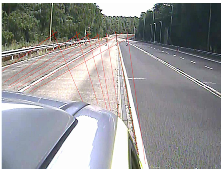
Figure 10: On-track calibration for fend parking angle
