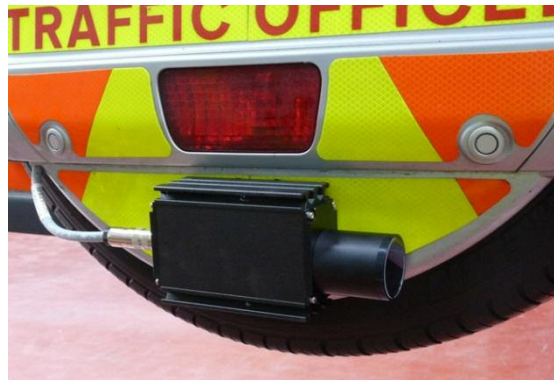
Figure 6: Laser distance measurement sensor, fitted to spare wheel cover on rear of TOV
