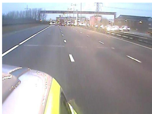
Figure 15: Live lane with TOV travelling forward; image as used to reorient the fender angle scale after camera movement
