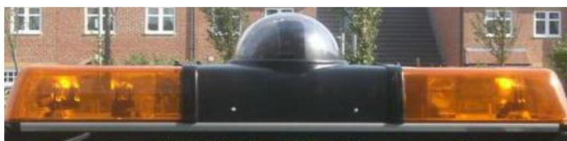
Figure 62: CCTV camera 'dome' integrated into Premier Hazard light bar
