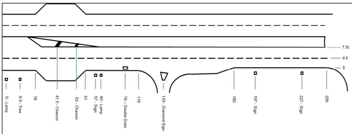
**Figure 12: Close up detail of approach road with distances from lamp on left (0) in metres (not to scale). Observation vehicle was parked roughly half way between lamp (0) and tree on left in single-car setup. Second car was parked just to left of lamp (0) in two-car setup**
