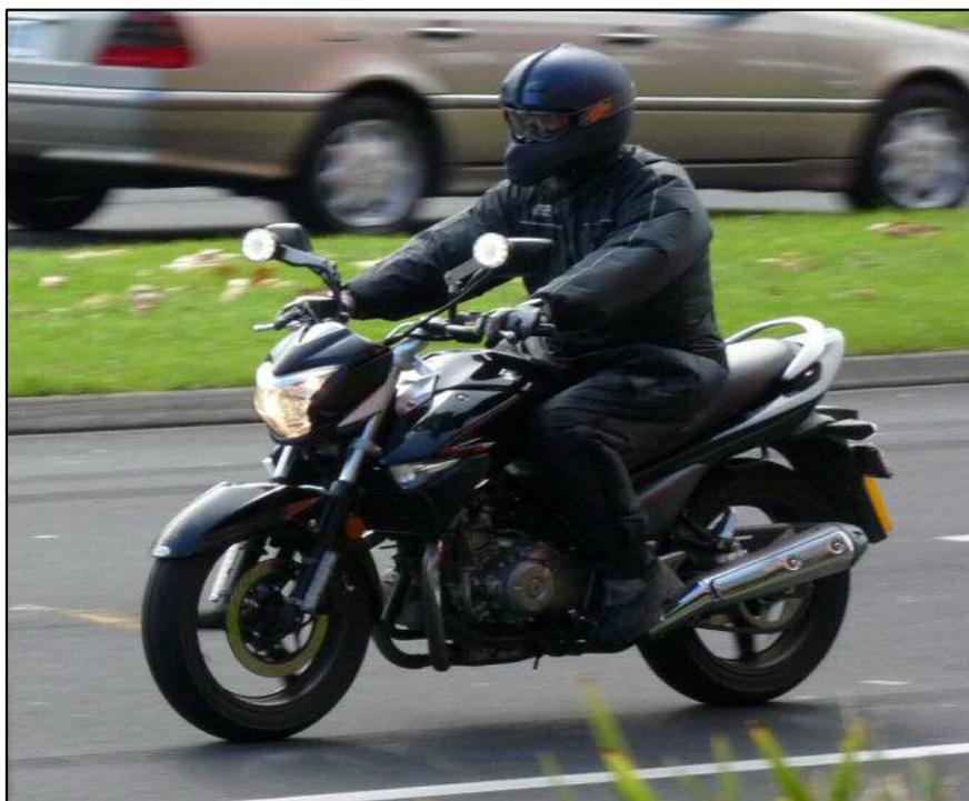
**Figure 10: Trials motorcycle, displaying upper DRLs ('V' configuration) with rider wearing black clothing and helmet cover**
