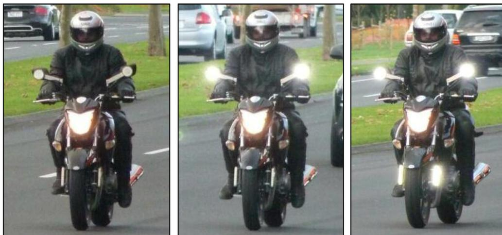
**Figure 9: Three lighting configurations; 'C' control, interventions 'V' and 'Y'**
