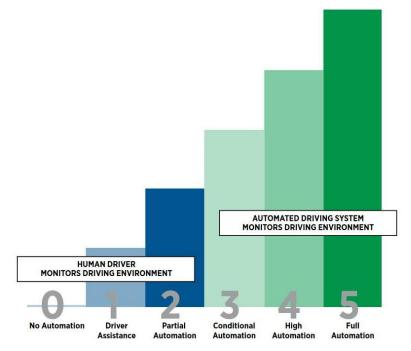
Figure 2: Six levels of driving automation (SAEJ3016, 2016)
