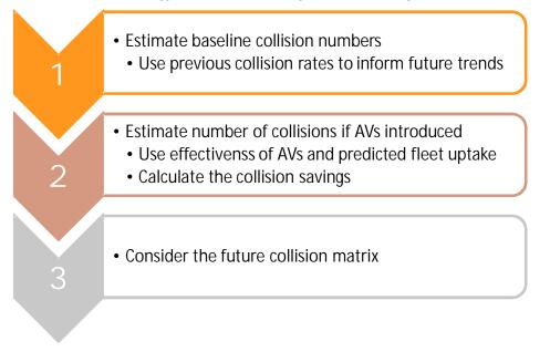
Figure 18: Overview of methodology for future collision modelling
