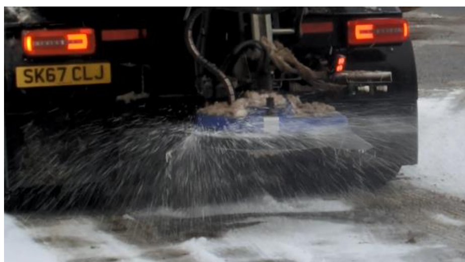
Figure 3. Brine distribution from spinner disc
