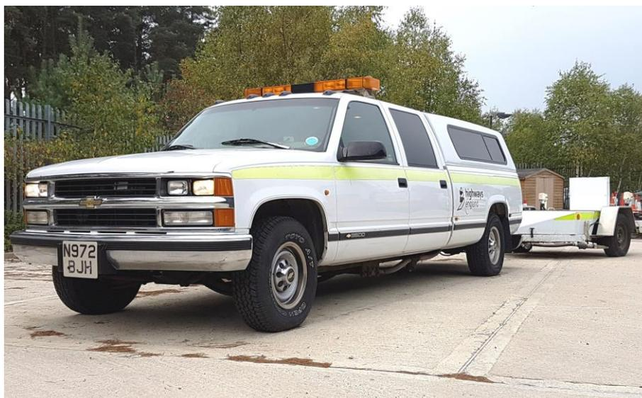
**Figure 2-1 The Pavement Friction Tester (PFT)**
