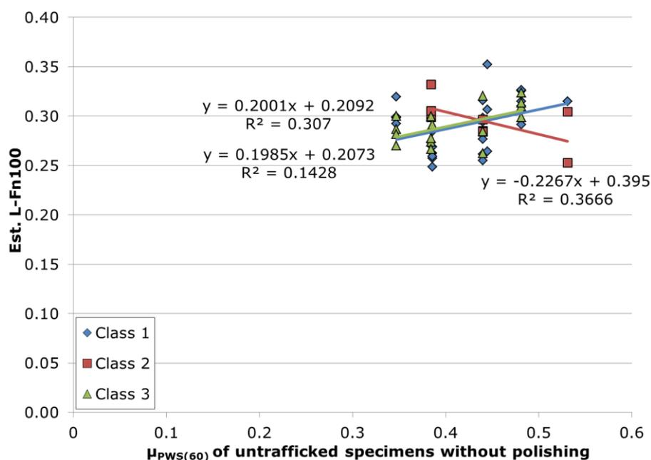
**Figure 5-12 Friction of master specimen Vs Est. L-Fn100**
