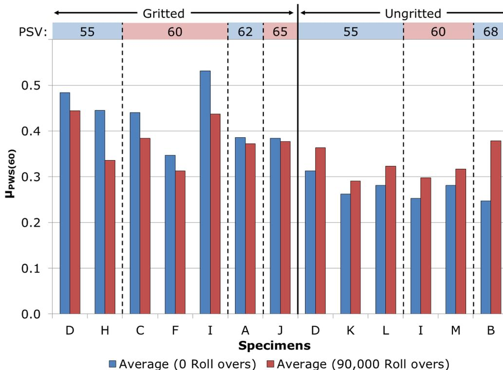
Figure 5-1 Average results of un-trafficked specimens after 0 and 90,000 roll overs
