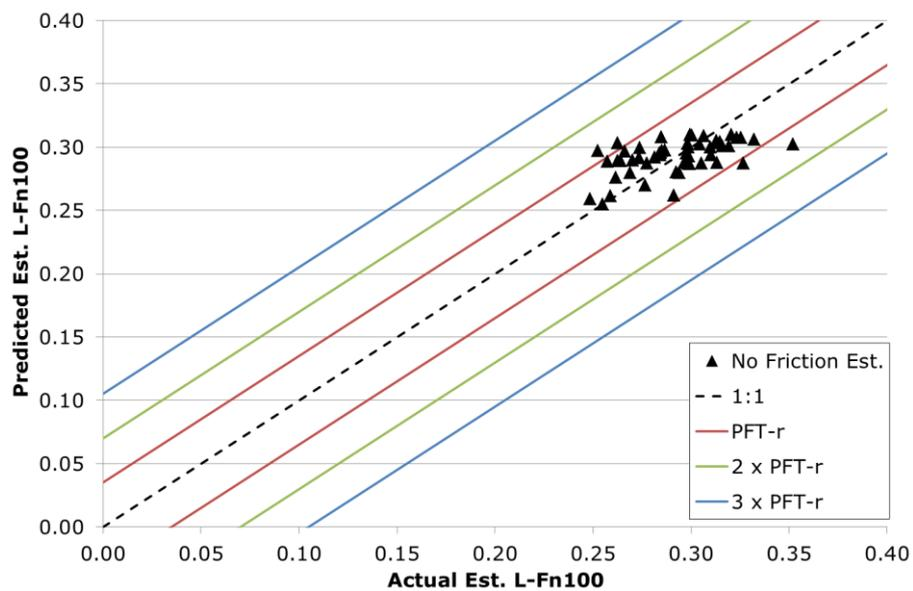
Figure 8-8 Predicted Vs. Actual Est. L-Fn100 values using no friction estimations
