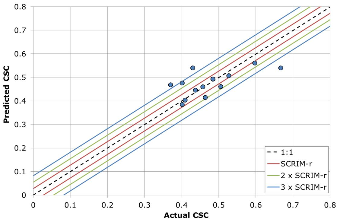
Figure 5-8 Predicted Vs Actual CSC for trafficked specimens (90,000 roll overs).
