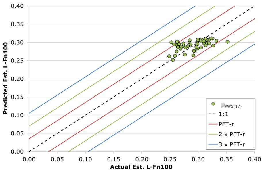
Figure 8-4 Predicted Vs. Actual Est. L-Fn100 values using  $\mu_{PWS(17)}$
