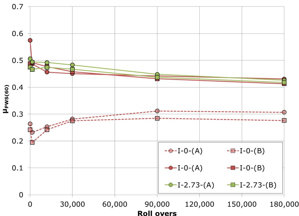
Figure 5-4 Wehner-Schulze machine results for material I<sup>6</sup>
