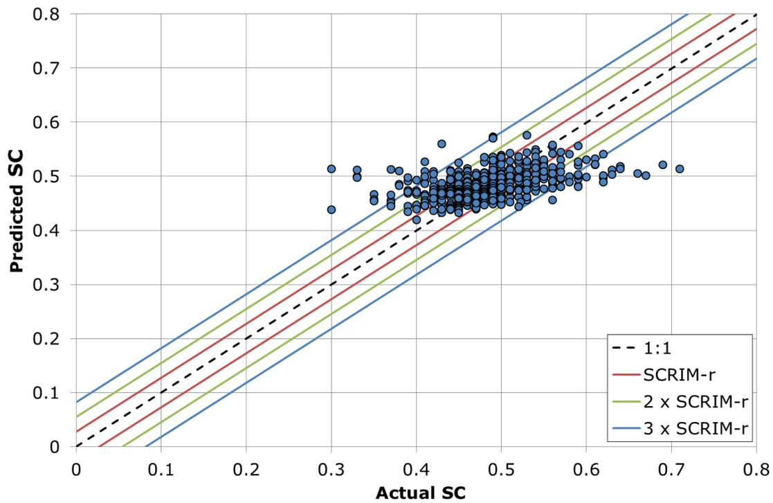
Figure 5-7 Predicted Vs Actual SC for all sections of TS network (90,000 roll overs).
