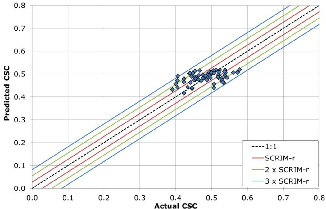
**Figure 5-9 Predicted Vs actual average CSC for materials ( zero roll overs)**
