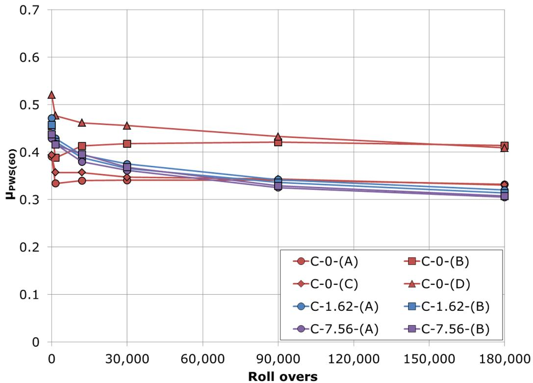
Figure 5-3 Wehner-Schulze machine results for material C<sup>5</sup>
