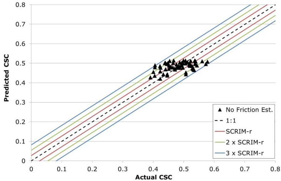
Figure 8-7 Predicted Vs. Actual CSC values using no friction estimations
