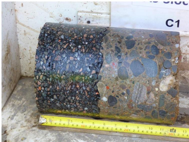
**Figure 2-1 Trafficked core extracted at site, TS2010 surface course to the far left**
