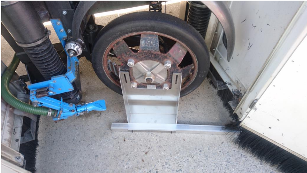
Figure 5.1 Test wheel angle equipment in use part 1
