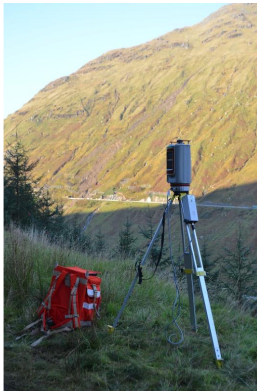
Figure 12 Riegl VZ4000 TLS being used from the forest track to scan the RabT slope
