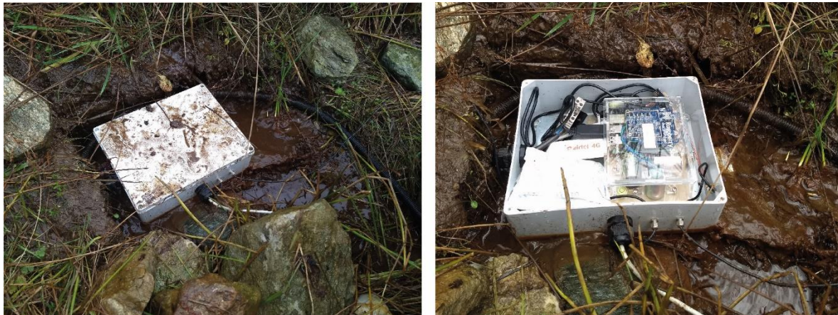
Figure 7 An example of one of the Raspberry Shake seismometer installations. The units are housed within an IP67 waterproof box with a separate battery box adjacent to the installation
