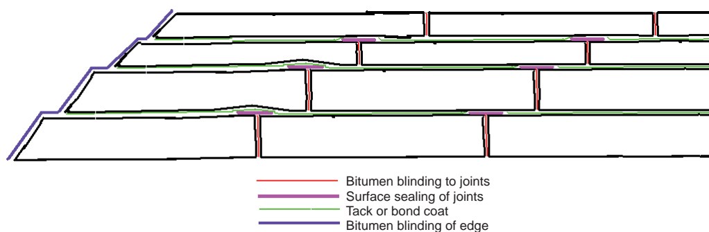
Figure 5.1 Overall sealing of all joints and edges in a pavement
