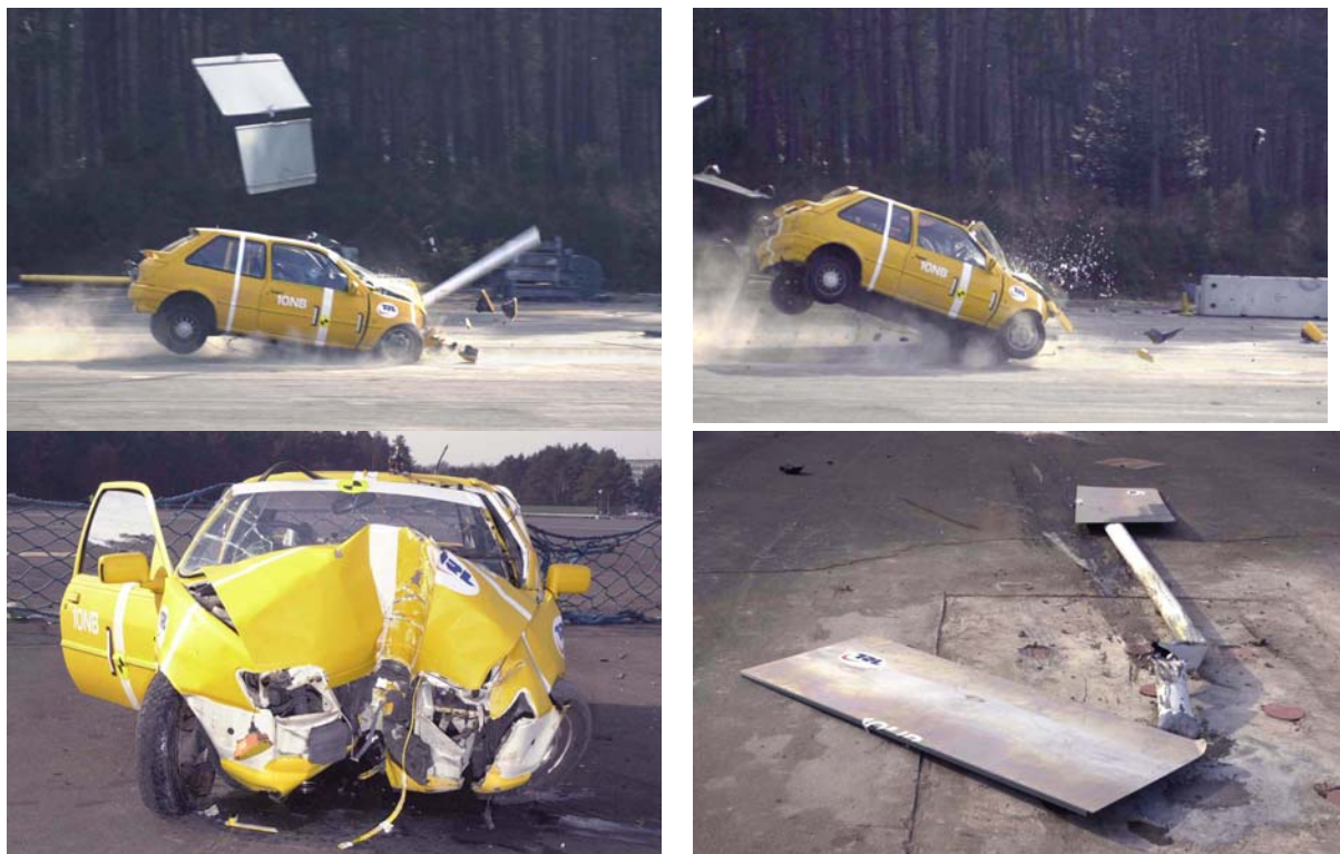
Figure 4: Testing of 114.3 mm diameter conventional signpost at 100 kph
