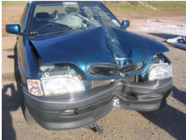
Figure 5: Vehicle following test at 100kph with a passively safe composite post
