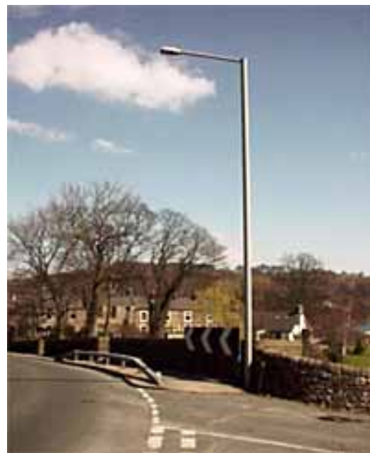
Figure 2: Passively safe lighting column
