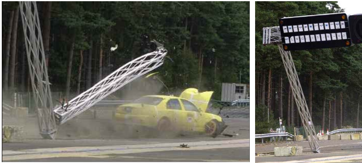
Figure 10: Test with lightweight sign and remaining leg after impact
