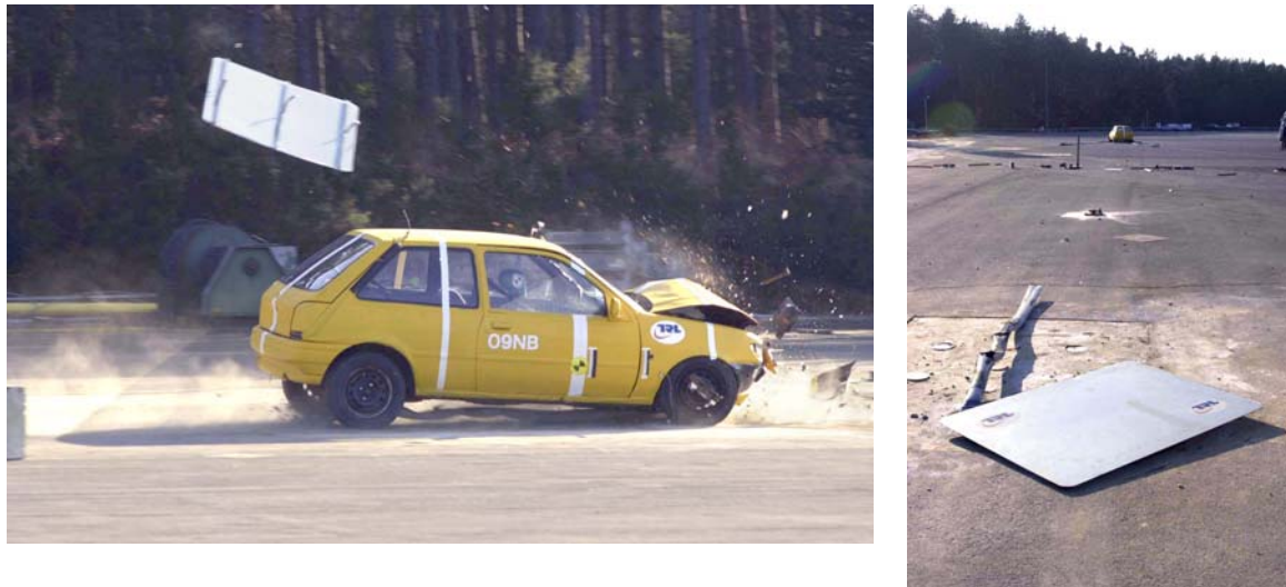
Figure 3: Testing of 88.9 mm diameter conventional signpost at 100 kph
