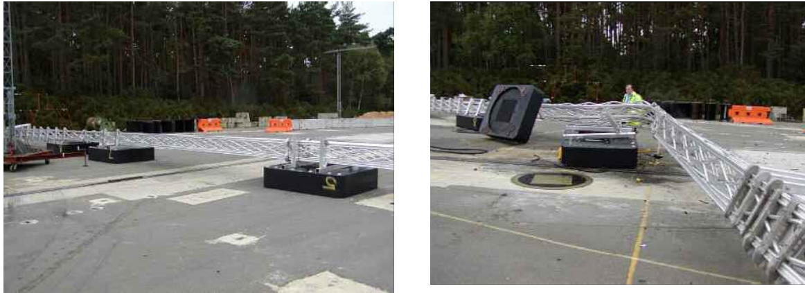
Figure 12: Transom before and after test with fallen gantry
