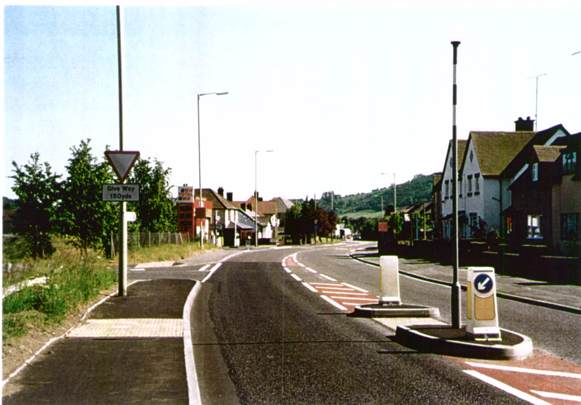
Fig 23. Pedestrian refuge and associated tactile paving on the footway and between the islands in the northern part of the village (looking south); the sign on the left gives advance warning of a requirement to give way at the White Meadow Close mini-roundabout
