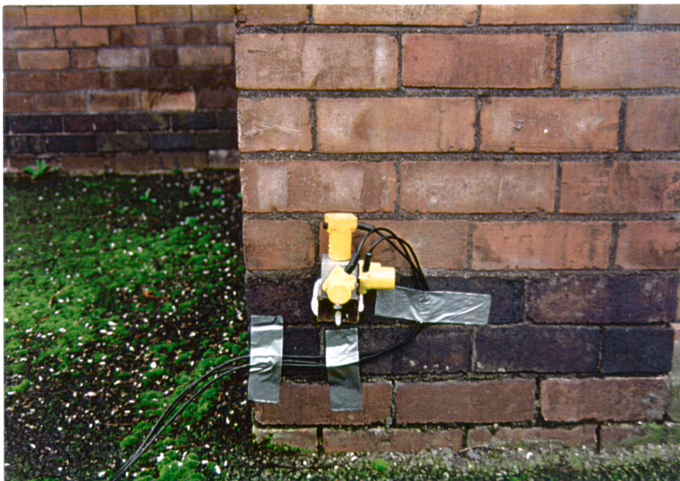
Fig 37. Triaxial geophone array attached to wall near ground level
