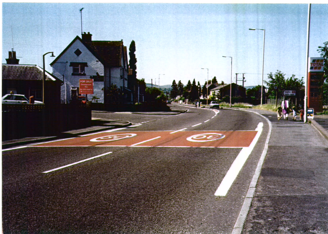
Fig 14. Repeated red patch with 30mph roundels north of the village centre (looking north)
