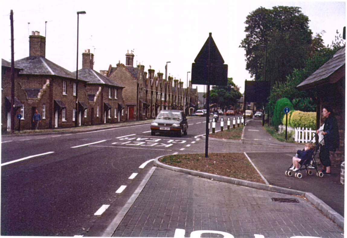
Fig.20 Kerb realignment to create horizontal deflection to traffic: kerb build-outs and sheltered bus bay opposite junction with Church Street, looking east (top) and similar features on other side of carriageway at drive to Thorney Park, looking east (bottom)
