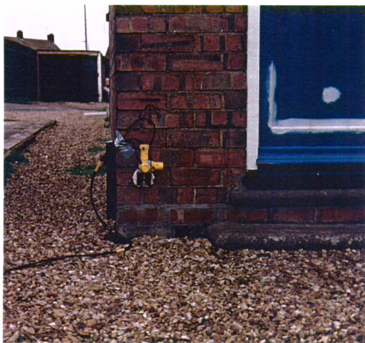
Fig.37 Installation of triaxial geophone array attached to wall near ground level
