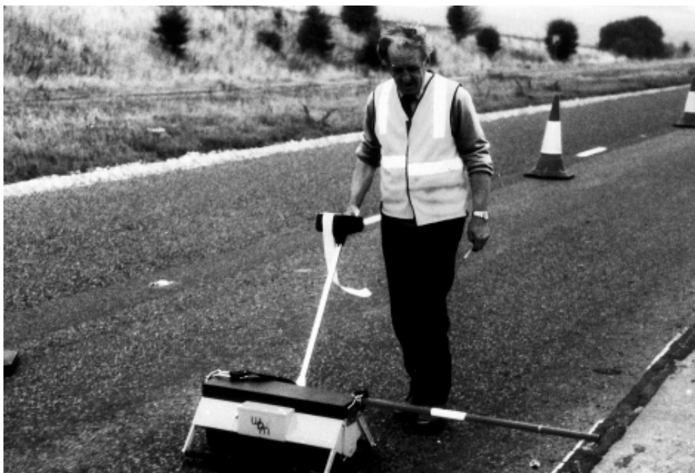
Figure 2 Location system in operation on TRL Mini Texture Meter
