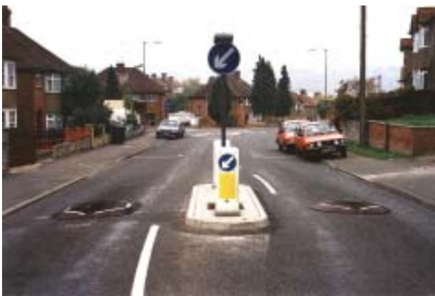
(e) Cushion pair at central island Chairborough Road (site 2) (Picture TRL)
