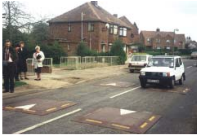
(b) Double-pair without buildouts or islands Muncaster (site 22) (Picture TRL)
