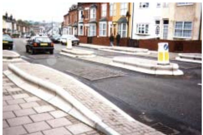
(f) Double-pair at refuge and pinch point Charles Road (site 31) (Picture TRL)
