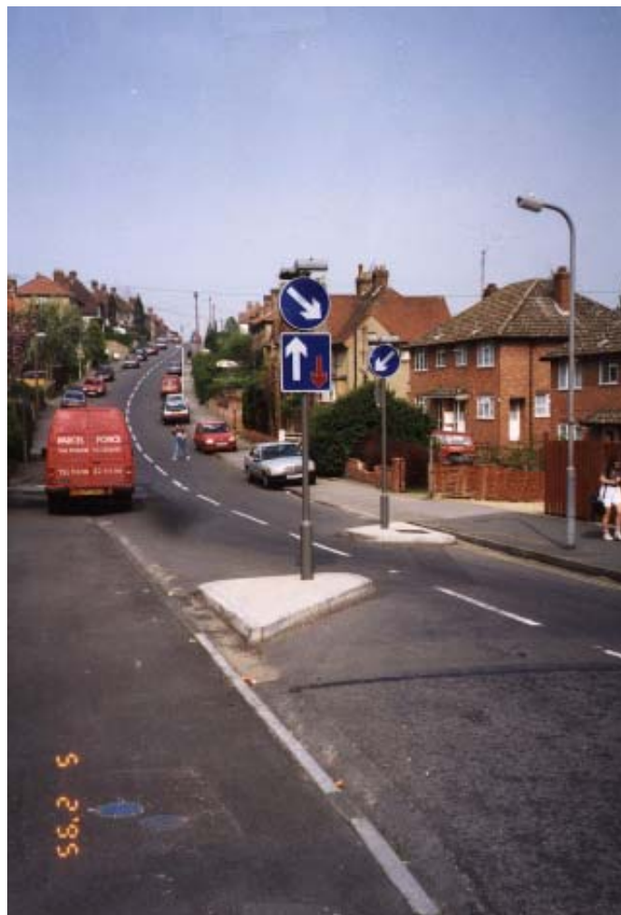
Plate 2 Example of a single lane working chicane: Scheme 5, Plumer Road
