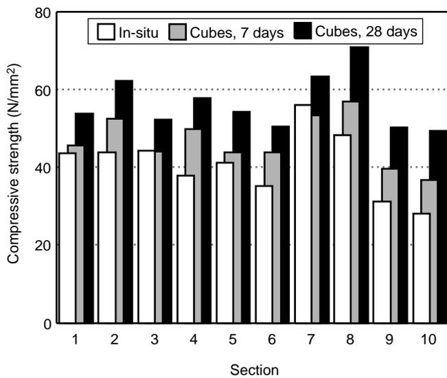
**Figure 2(a)** Compressive strength of cubes cured at 20°C compared to in-situ strength
