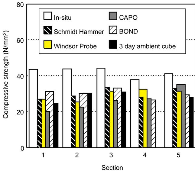
**Figure 4** Compressive strength from 3-day near-to-surface tests compared to 3-day ambient cubes and 28-day in-situ strength
