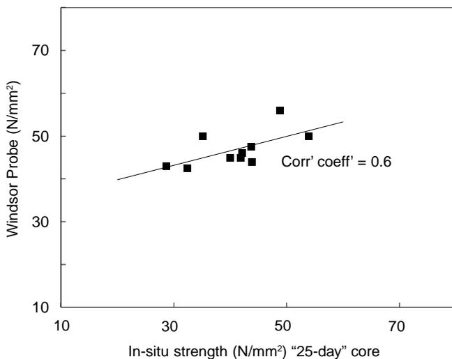
**Figure 7** Linear regression analysis Windsor Probe (penetration resistance) 28-day test (Sections 1–10)
