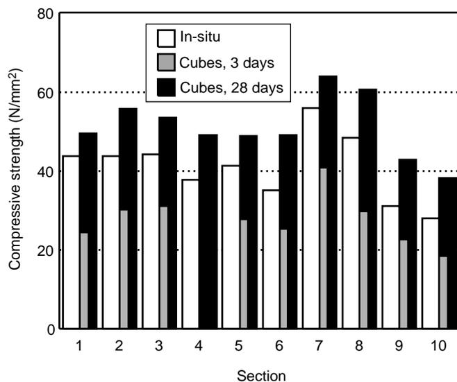
**Figure 3** Compressive strength of cubes cured at ambient compared to in-situ strength
