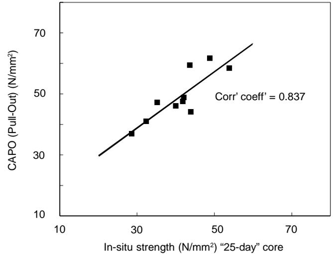
**Figure 8** Linear regression analysis CAPO (pull-out) 28-day test (Sections 1–10)
