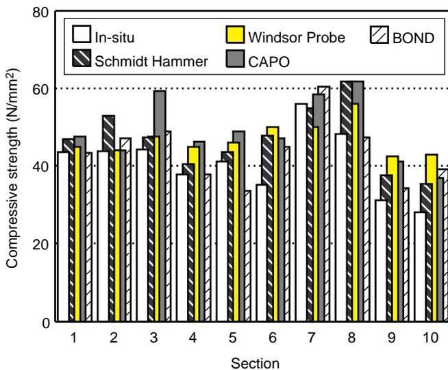
**Figure 5** Compressive strength from 28-day near-to-surface tests compared to 28-day in-situ strength
