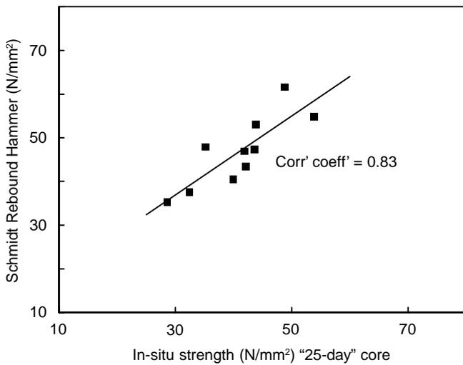
**Figure 6** Linear regression analysis Schmidt Rebound Hammer 28-day test (Sections 1–10)
