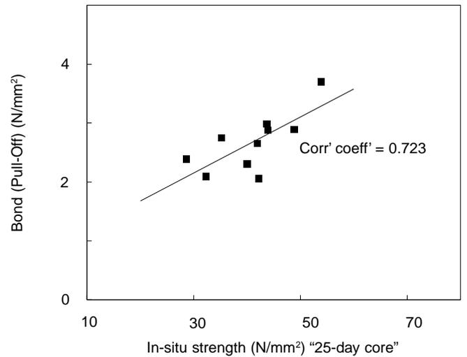
**Figure 9** Linear regression analysis BOND (pull-off) 28-day test (Sections 1–10)
