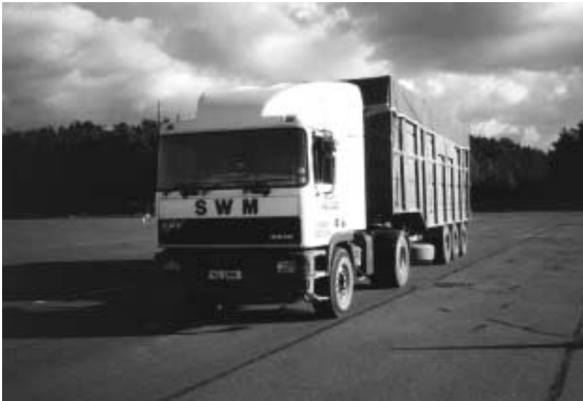
Plate 11 Test vehicle 4 (tractor and tipper trailer, steel suspension — unladen)
