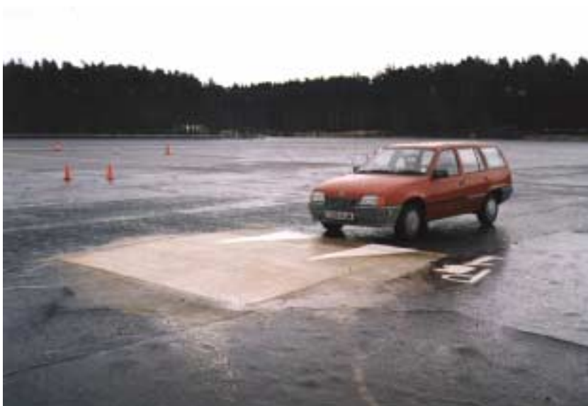
Plate 1 Profile P1, sinusoidal hump, 3.7m long
