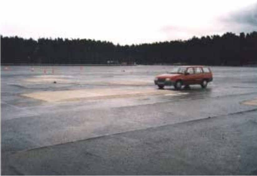
Plate 4 Profile P4, flat-top hump with sinusoidal ramps
