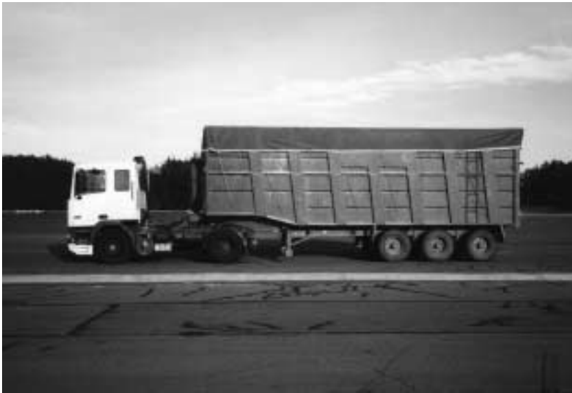
Plate 8 Test vehicle 1 (tractor and tipper trailer, air suspension — laden)
