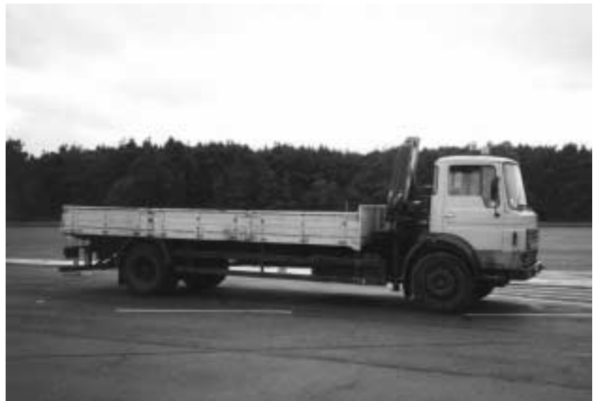
Plate 12 Test vehicle 5 (dropside rigid truck, steel suspension — unladen)
