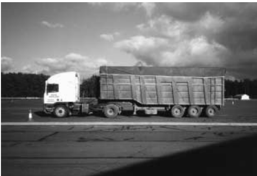
Plate 10 Test vehicle 3 (tractor and tipper trailer, steel suspension — laden)
