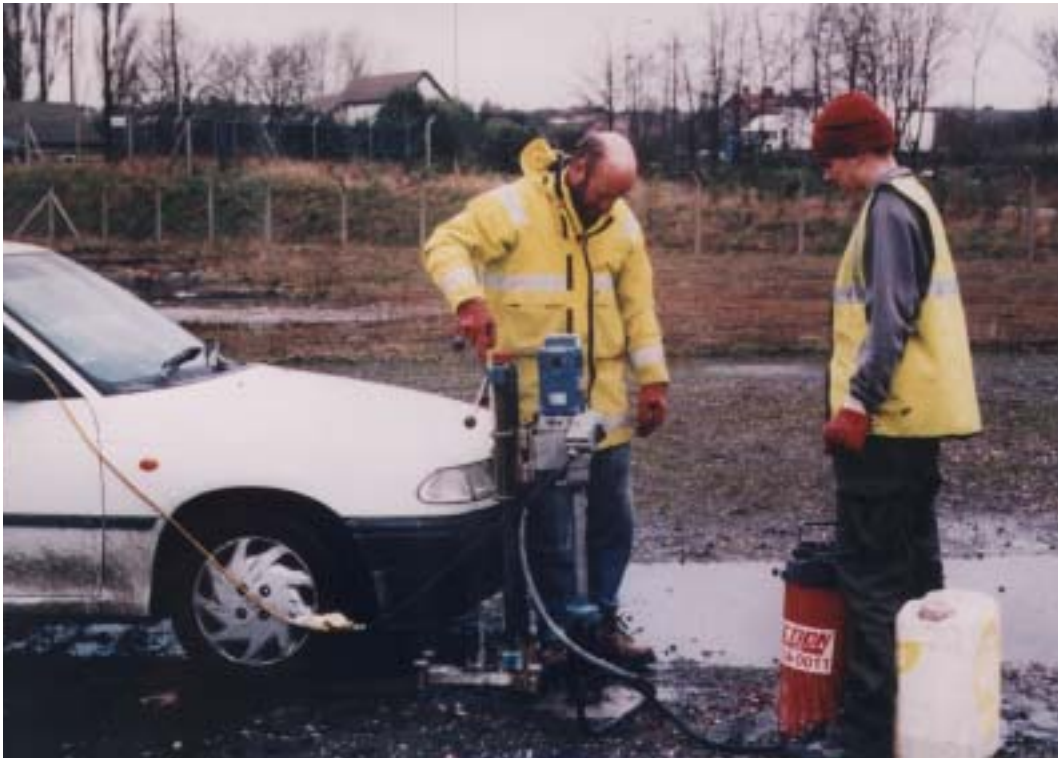
Plate 3 Drilling of Phase 2 core samples
