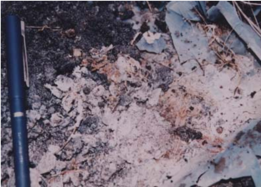
Plate 5 Calcareous precipitate from material D slab
