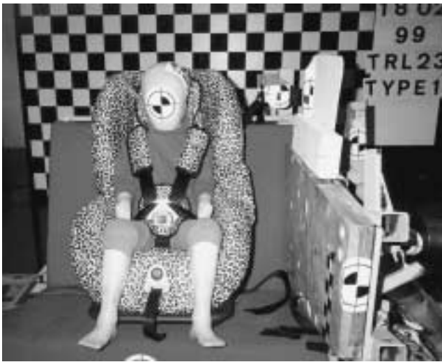
Figure 12 CRS positioning on test seat
