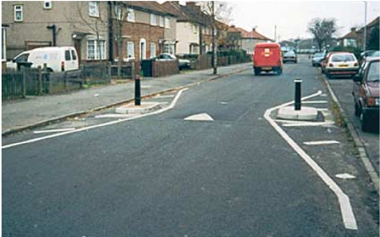
Figure 11 Combined pinch point and speed cushion: Broadmark Road, Slough
