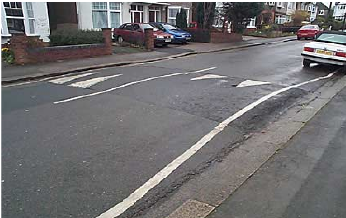
Figure 7 Round-top road hump: Milton Road, Sutton
