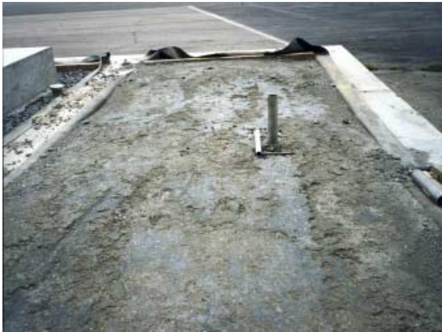
Plate 5 Test bed of contaminated silt treated with lime (sample being taken for triaxial testing)
