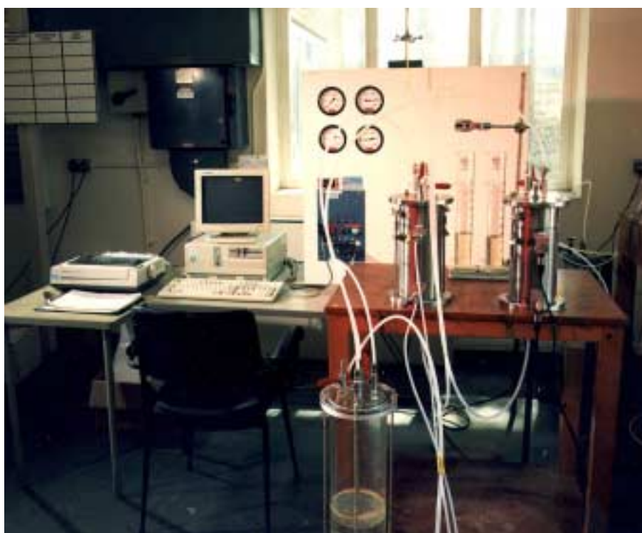
Plate 4 Apparatus for dynamic leaching tests in the laboratory
