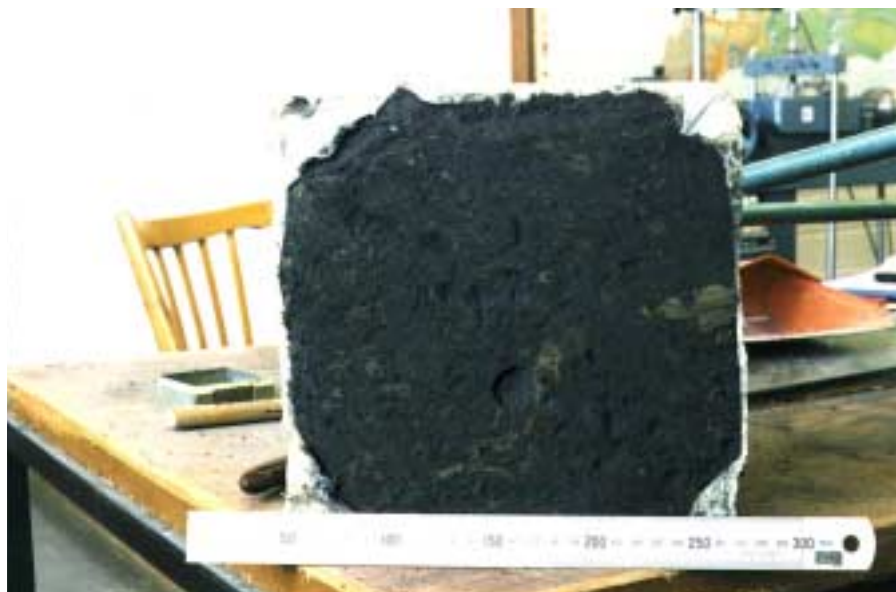
Plate 1 Block sample of lime modified silt from A13 three years after construction
