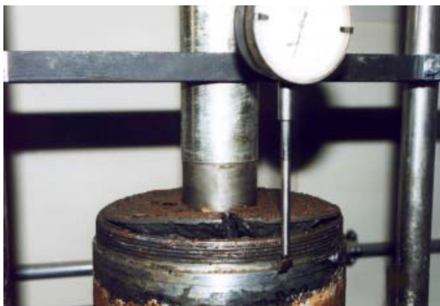
Figure 14 CBR test showing failure surface
