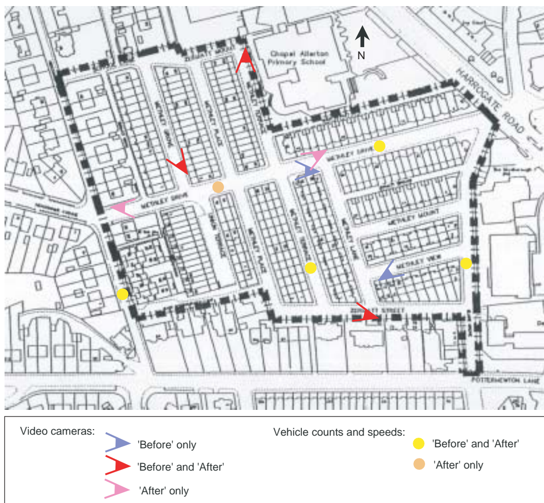
Figure 4.1 The Methleys Home Zone – site locations for automatic vehicle counts / speed measurements and for fixed video cameras
