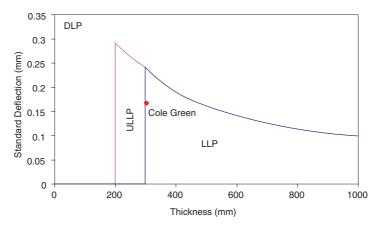
Figure A.3 The 85th percentile of deflectograph results at Cole Green compared to the criteria given in Figure 3.1
