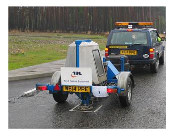
Figure 4.1 The falling weight deflectometer (FWD)
