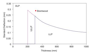
Figure A.1 The 85th percentile of deflectograph results at Brentwood compared to the criteria given in Figure 3.2
