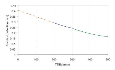
Figure 4.3 Extrapolated deflection-thickness criteria for determining 'excess' thickness
