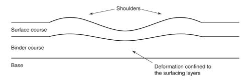
Figure 5.2 Illustration of the cross-section of a typical non-structural rut
