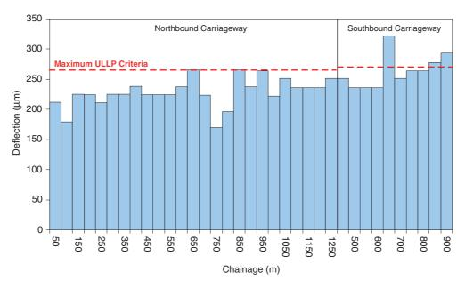
Figure A.5 85th percentiles of deflectograph measurements at Snodland
