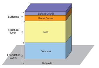
Figure 2.1 The layers of a long-life flexible pavement
