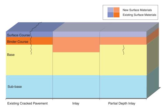
Figure 6.3 Illustration of partial depth inlay treatment
