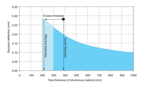
Figure 4.2 Illustration of 'excess' thickness
