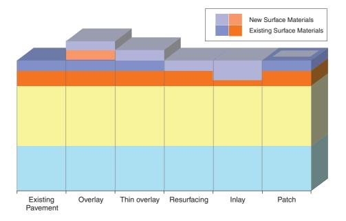
Figure 6.1 Types of treatment permitted for long-life pavements
