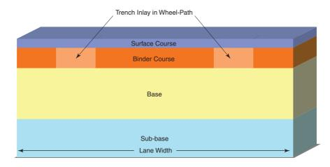
Figure 6.2 Illustration of trench inlay treatment
