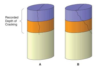
Figure 5.1 Illustration of cores showing different paths of crack propagation
