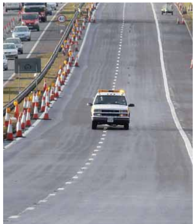
Figure 9.12 The PFT making a test pass to measure dry friction at 20 km/h
