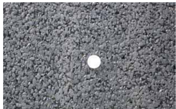
Figure 8.4 0/6mm SMA gritted (left) and ungritted (right)
