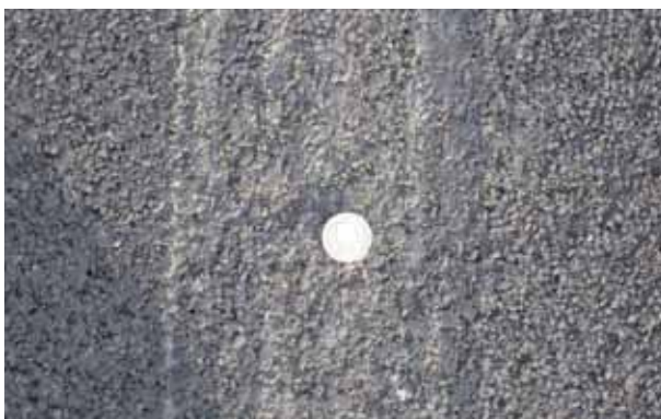
Figure 8.4 0/6mm SMA gritted (left) and ungritted (right)
