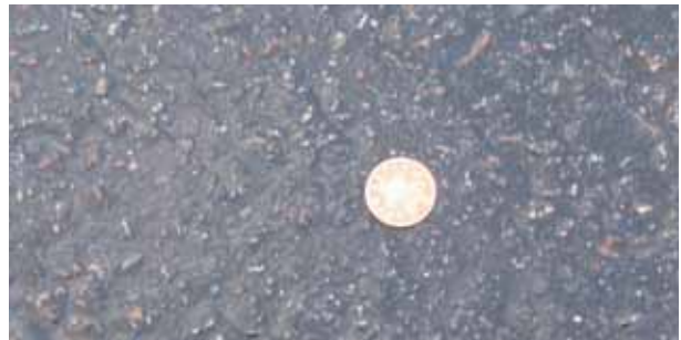
Figure 3.8 Low surface texture depth (Site TSMA6)
