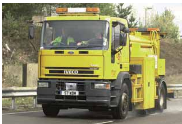
Figure 8.1 The SCRIMtex measures the SFC and SMTD
