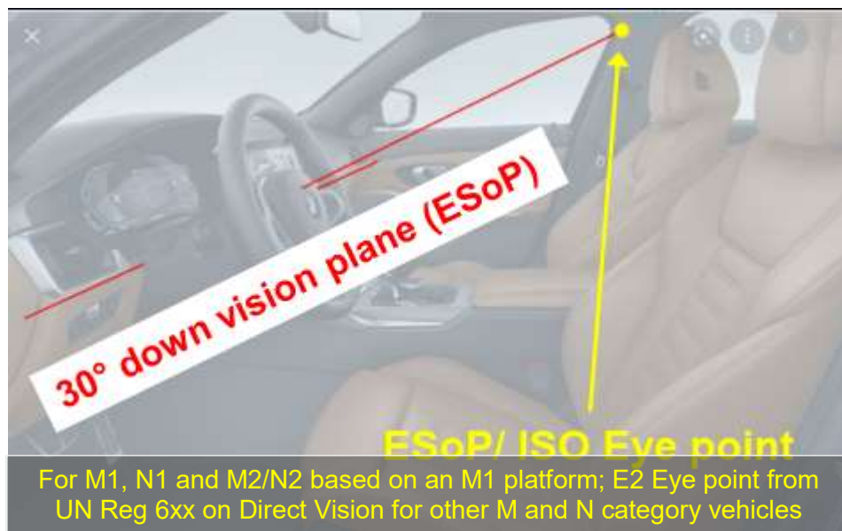
Figure 1: Illustration of 30° downward vision plane for an M1-category vehicle (based on a figure provided by ACEA)
